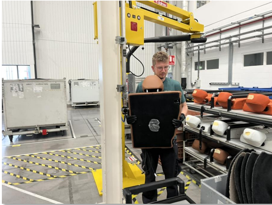
Figure 5 - Example of lifting part from Trolley (Author, 2025)
