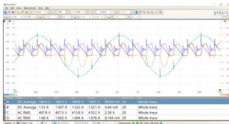
Figure 29 - Practical - Pico Scope Discontinuous Current 1000rpm
