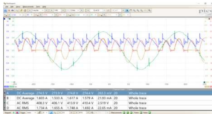
Figure 32 - Practical - Pico Scope Discontinuous Current 1500rpm
