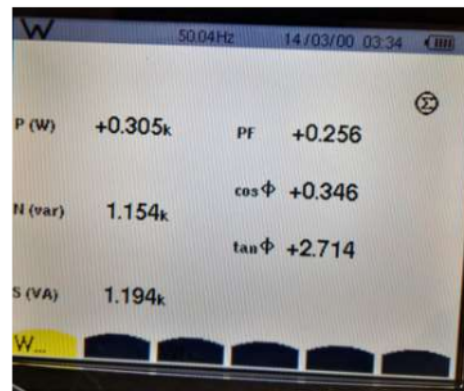
Figure 31 - Practical - Power Analyser Discontinuous Current 1000rpm
