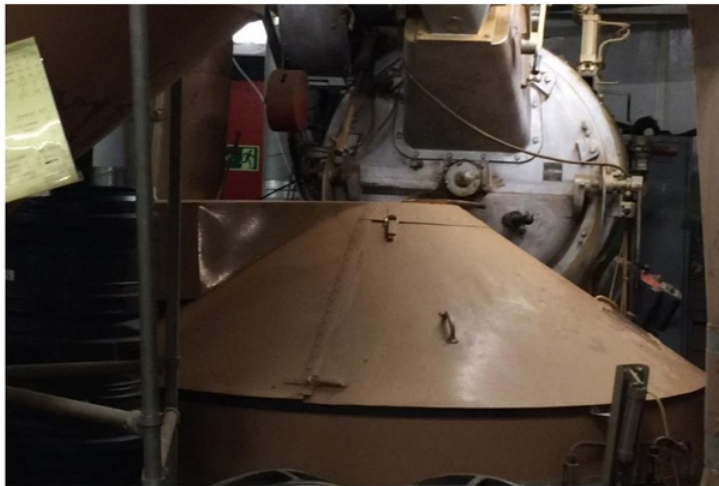
Figure 7: Shows the cooling bed used to cool the roasted beans.
