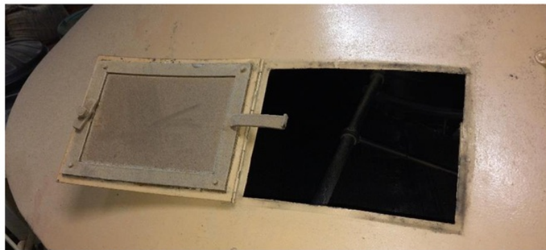
Figure 9: Shows how moving parts can be accessed during operation through the hatch.
