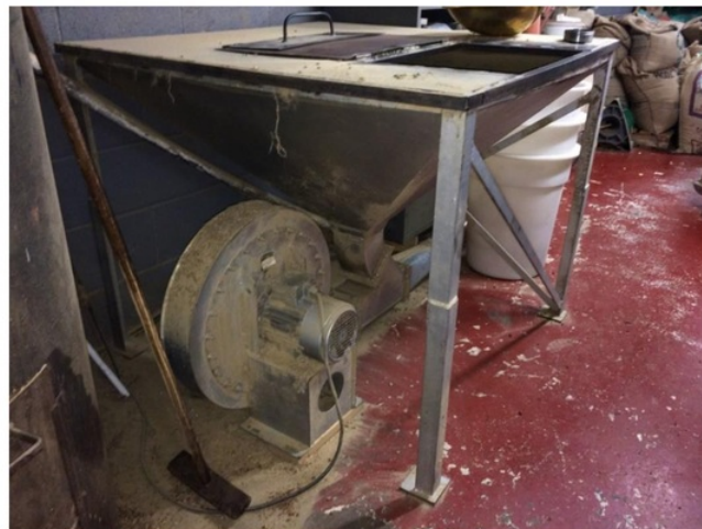
Figure 2: The hopper and blower for the raw beans, the start of the process.
