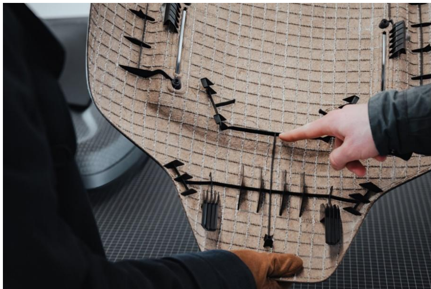
Figure 20 Bcomp panel made from sustainable materials with integrated reinforcement to improve stiffness and strength (Bcomp).
