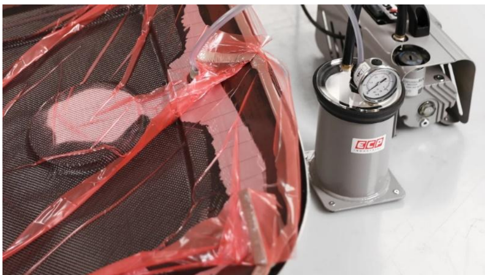
Figure 5 Vacuum infusion manufacturing set-up used to produce the composite specimens, showing dry fibre lay-up, vacuum bagging, and infusion equipment prior to resin flow (Easy Composites Ltd).
