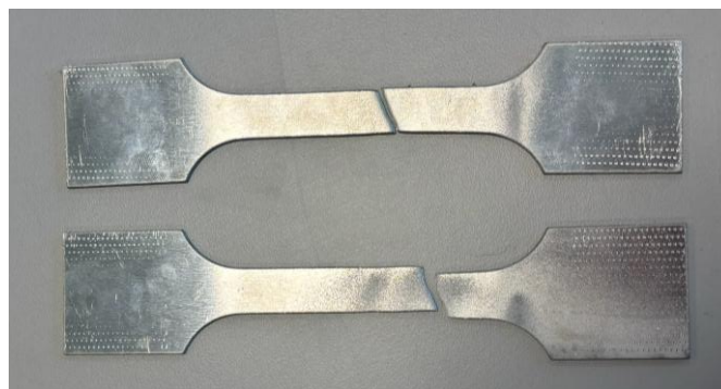
Figure 7 Showing the two aluminium samples, both showing similar failure modes.
