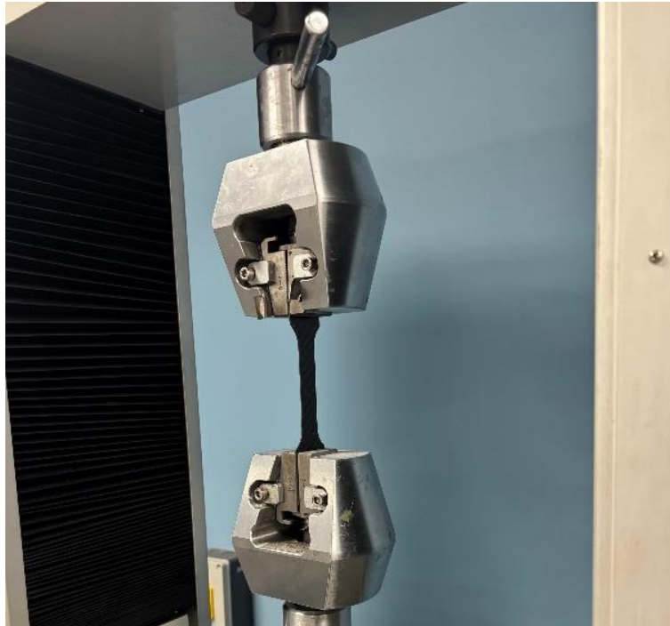
Figure 4 Carbon specimen mounted in the Denison prior to the extensometer being placed on and then tested.
