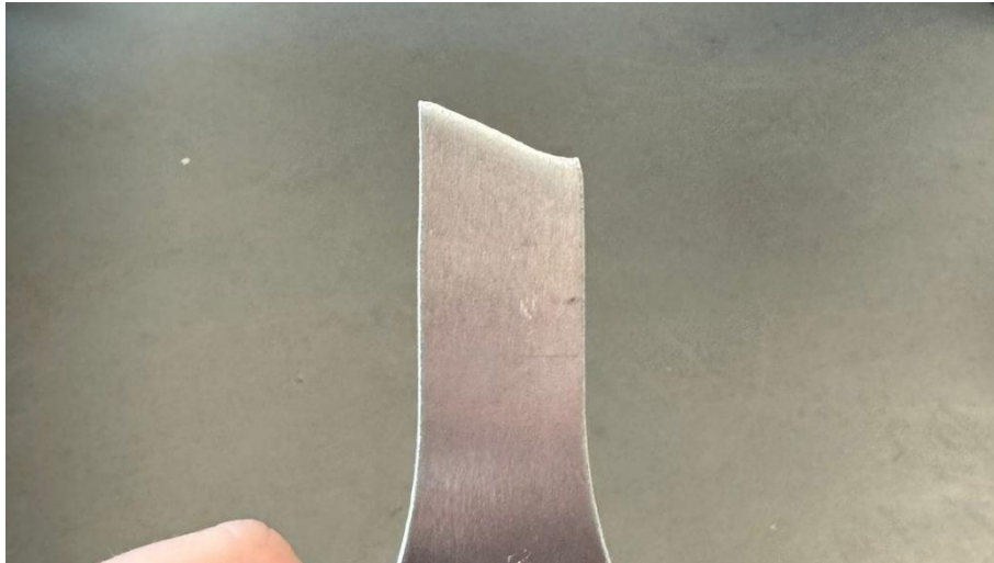
Figure 6 - Aluminium Sample Necking
