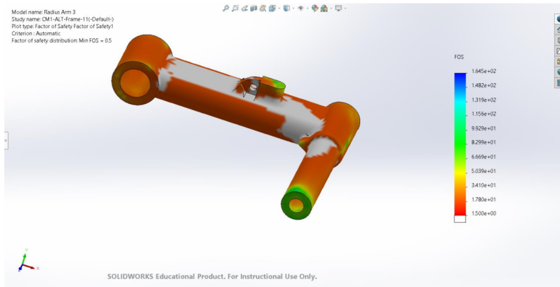
Figure 21 Model redesign 3 - Factor of Safety
