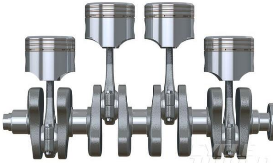
(Figure 3: Flat-Plane Crank Assembly (Cycle World, 2015))
