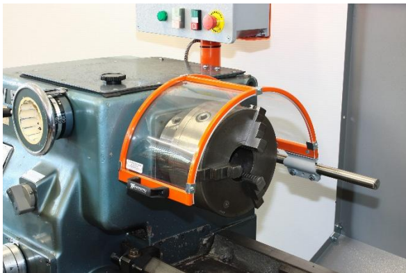
Figure 1- Lathe Guard (Solon Systems 2025)
