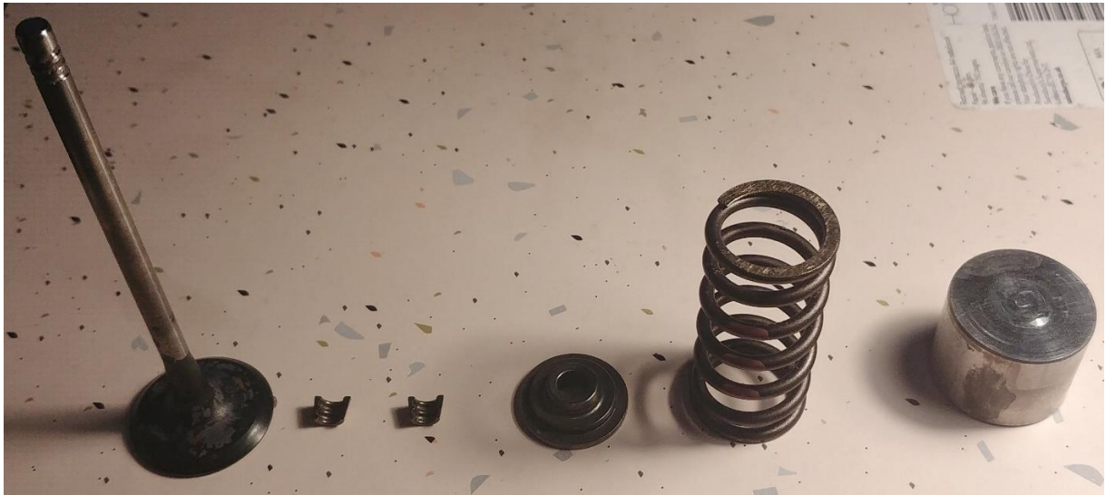
Figure 2-1: Reciprocating Valvetrain Components
