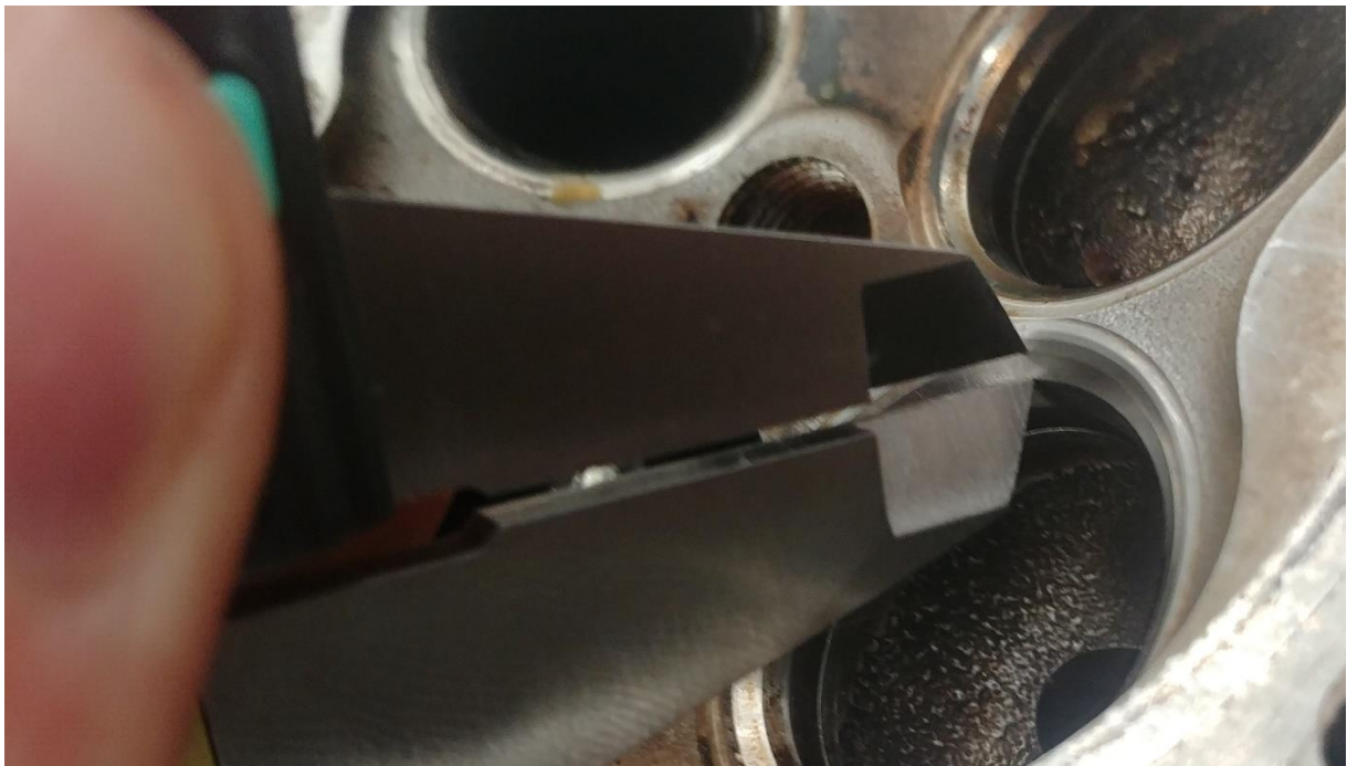
Figure 2-2: Valve Seat Measurement
