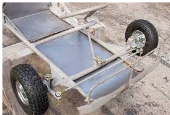
Figure 8: steering solution for soapbox
