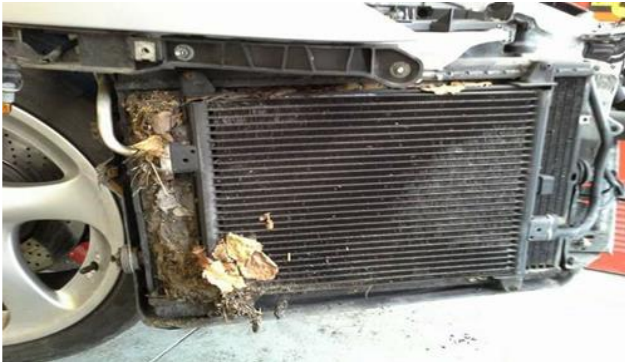
The picture above shows the real world example of debris build up on Porsche 911.
