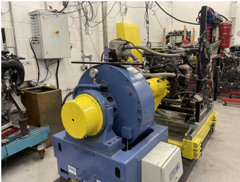
Figure 2-1 Photograph of Engine Dynamometer (F. Flye, 2025)
