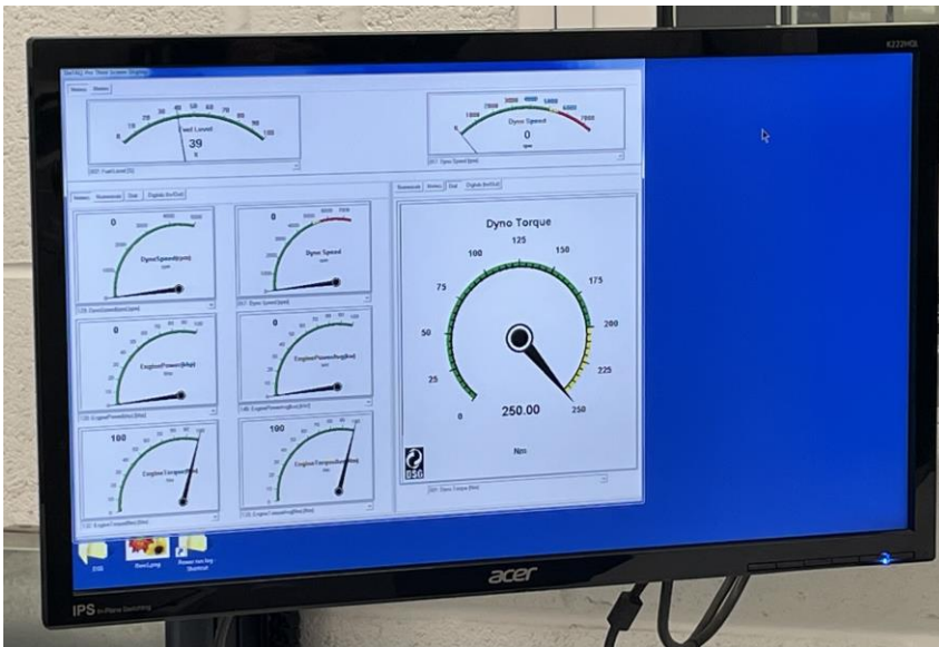
Figure 2-4 Photograph of the Dynamometer/ Engine speed and torque (F. Flye, 2025)
