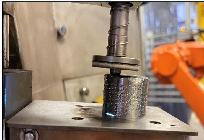
Figure 21 - Poorly positioned CRM on electrode
