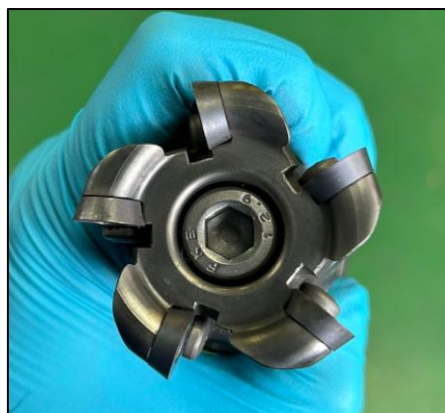
Figure 27 - Spare Miller head with new tips
