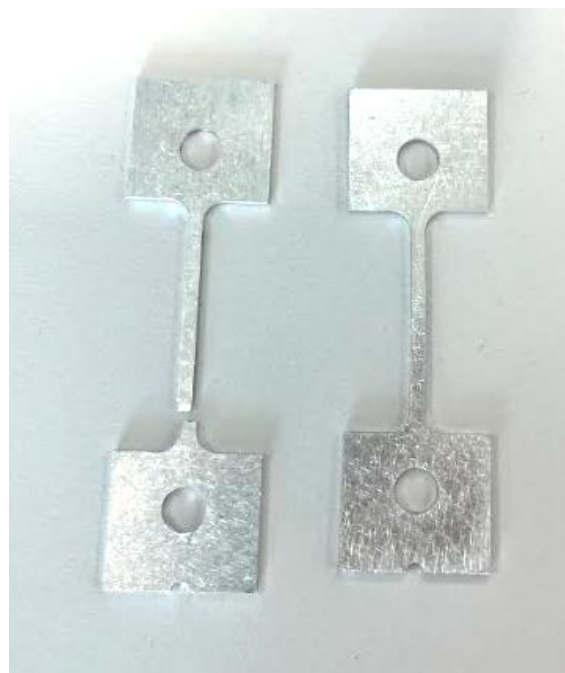
Figure 8 Comparison of Broken and New Specimen
