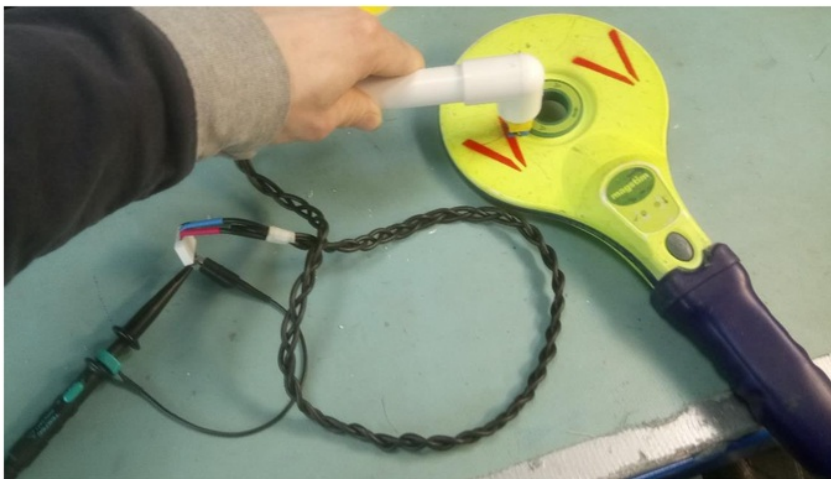
Figure 8 - Search coil measuring magnetic field with scope output
