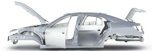
Figure 10: An image to show a modern aluminium monocoque chassis, designing the chassis as integral with the body (Haomei Auto Aluminium – 2025).
