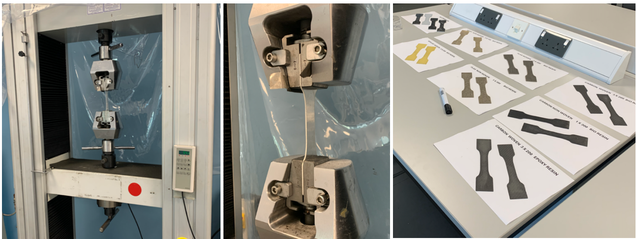
Figure 12: Universal Testing Machine (UTM), used to evaluate the tensile strength and failure of different materials (Burnside, R. – 2025).
