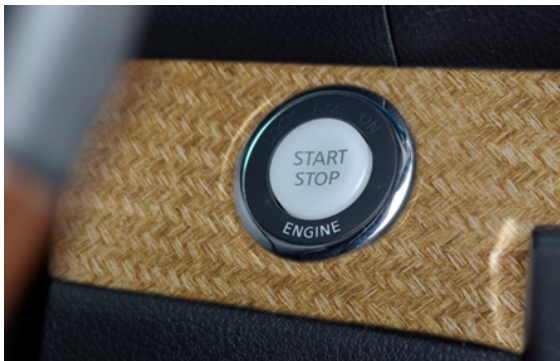
Figure 8: An example of Flax, woven into a fibre mat to be “thermo-compressed and injection moulded.” (Nehls, G. - 2022)
