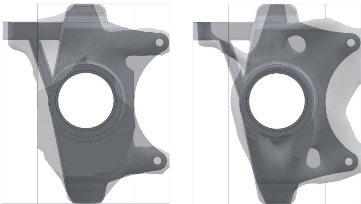
Final optimized upright overlaid with second topology study (left) and final topology study (right)
