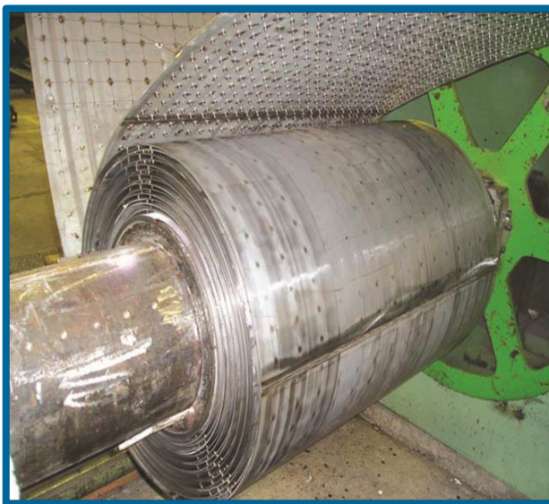
Figure 33: Manufacture of the SHE heat-transfer body (Andersson, 2008)
