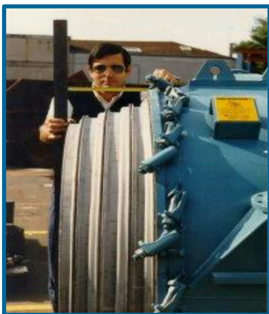
Figure 37: SHE de-pressure failure (Alfa Lava, ndl)
