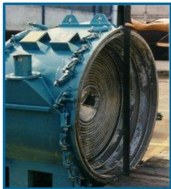
Figure 37: SHE de-pressure failure (Alfa Lava, ndl)
