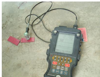
Figure 1. Pulse-echo ultrasonic testing experimental set up
