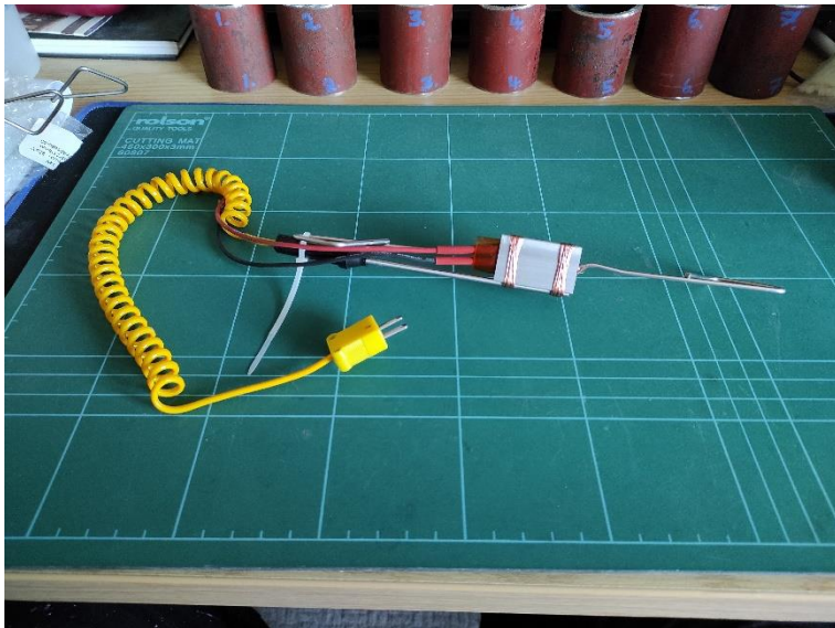
Figure 10.7 PTC element and thermocouple assembly
