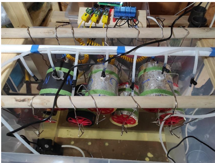
Figure 10.5 Water distribution system in place within environmental tank.
