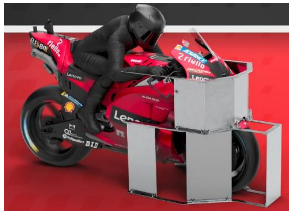
Figure 6 - MotoGP Regulation Check (MotoGP,2022)
