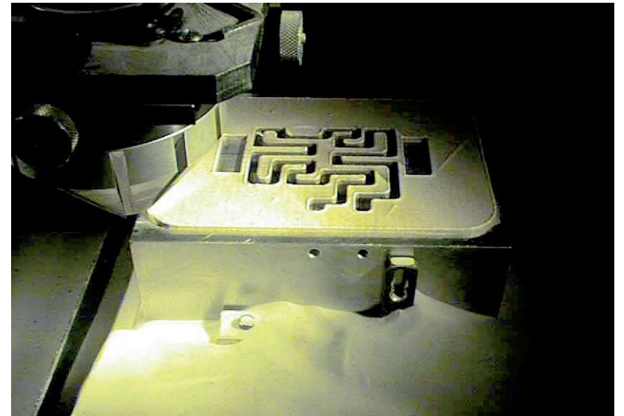
LENS, cavity during the construction process (Source: Optomec)
