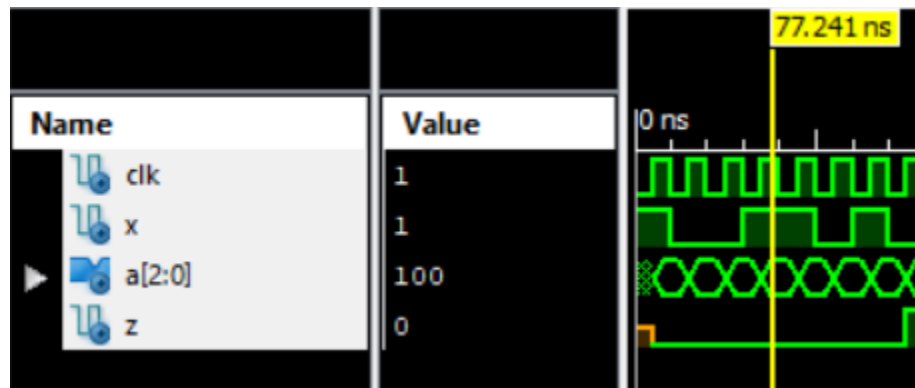
Figure 46 - FSM VHDL, Simulation, Transition D/011 to E/100
