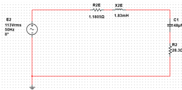
Figure 14: Voltage Regulation Overload Equivalent Circuit
