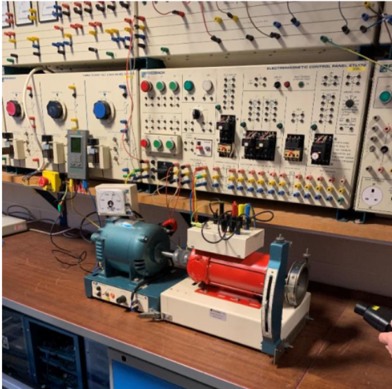
Figure 23: Motor practical setup
