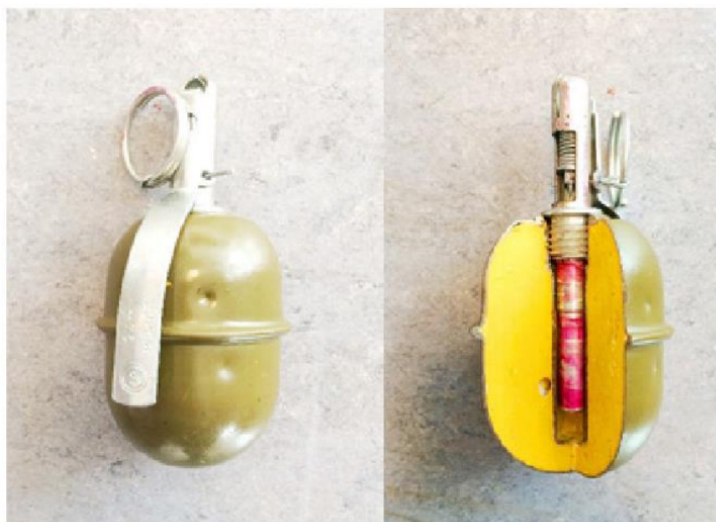
Figure 9 - Sectioned view of RGD-5 grenade [6]
