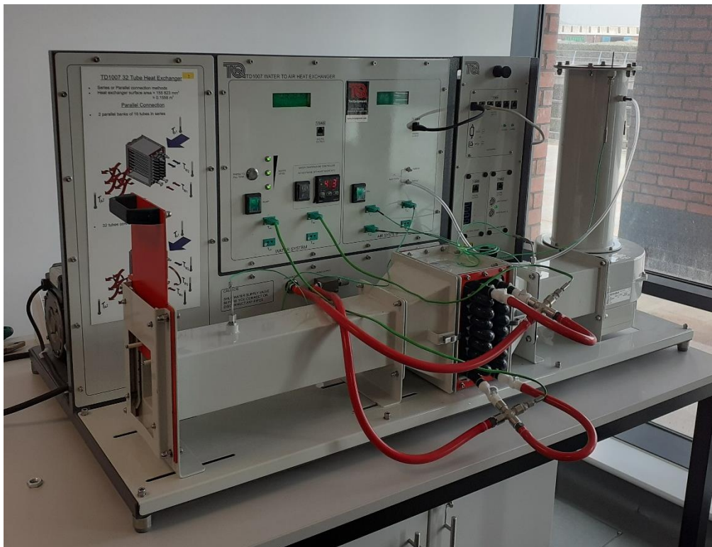
Figure 1 - Picture showing the TD1007 water to air cross-flow heat exchanger used in the experiments.
