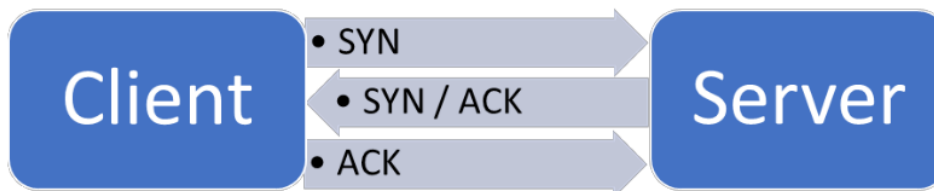
Figure 3: SmartArt representation of three-way handshake.
