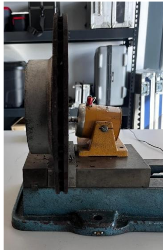
Figure 5 Amplifier Actuator which taps the brake disc (the specimen)
