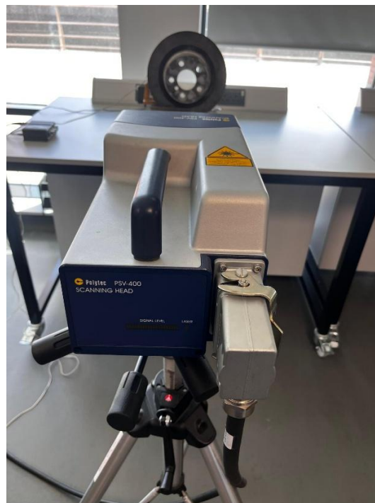
Figure 11 Polytec Scanning Head PSV-400 & Brake Disc
