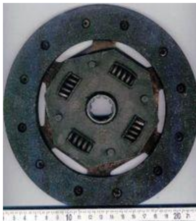
Single, dry, clutch friction disc. The splined hub is attached to the disc with springs to damp chatter
