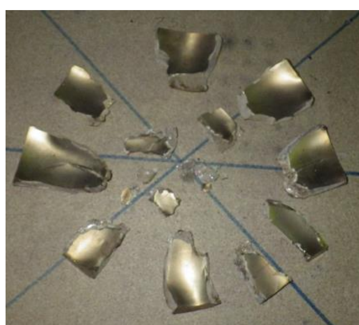
Figure 3: The physical results from the first firing using 75g of PE8 with the component and charge submerged in water. It is clearly visible that shape destruction of the component was achieved.
