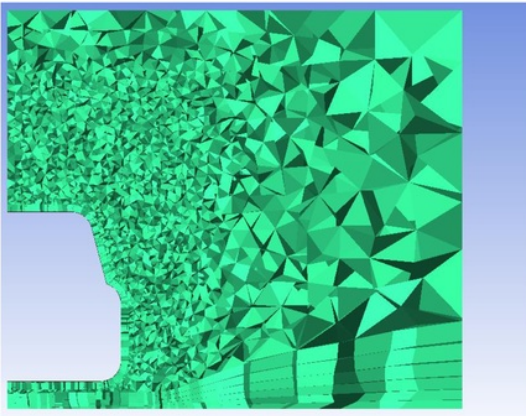
Figure 3-2, Example of a Delaunay Mesh
