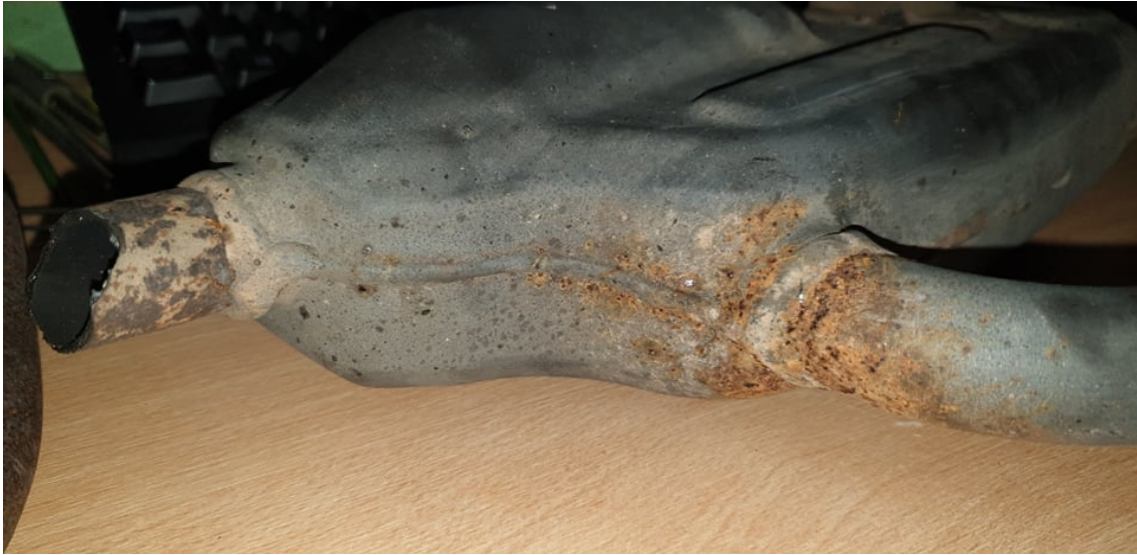
Figure 2: Catalytic converter and broken header pipe.
