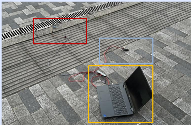
Figure 2 - Full stack deployed. The red box outlines the MKR 1010 board with HC-SR04 sensor; the blue box is the eduroam NAT gateway running on an ESP32 Nano S3; and the yellow/orange box shows the developer laptop running the C.D.S.W detection suite
