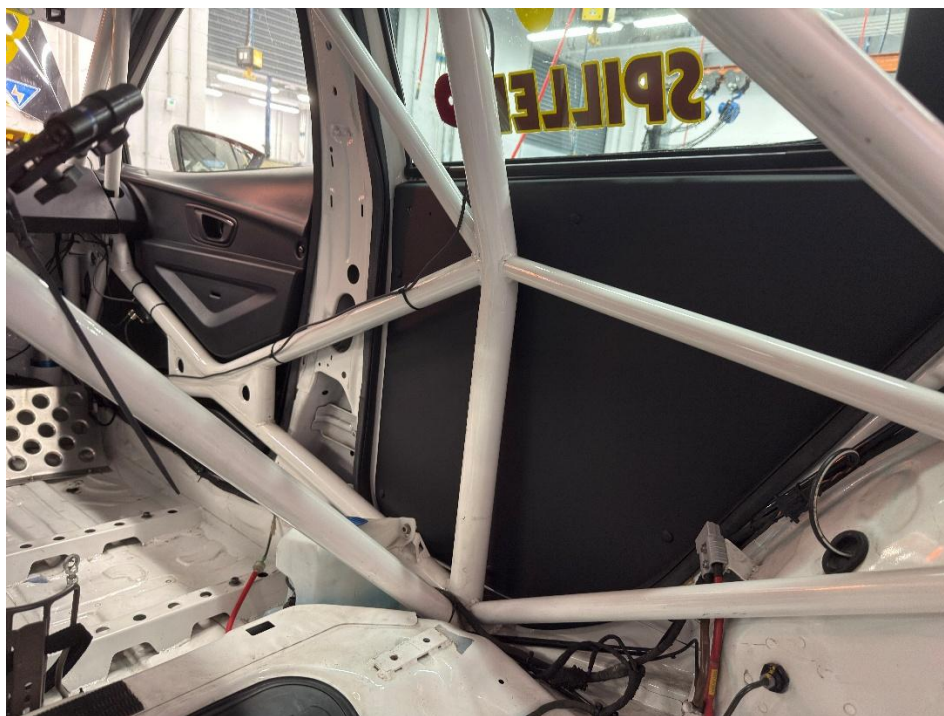
Figure 7 Rear door structure showing local modification and lightweighting for race use
