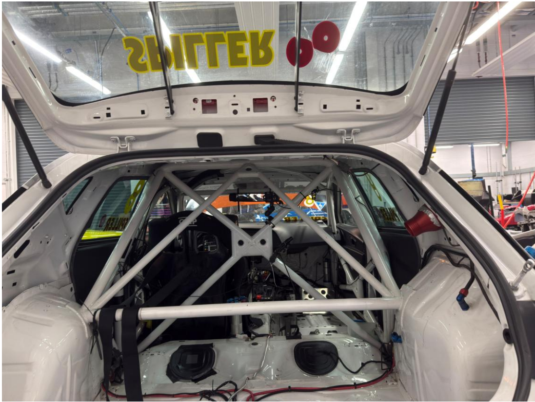
Figure 3 Overall roll-cage layout showing integration with the production-based bodyshell
