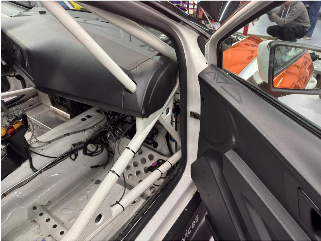
Appendix Figure A1 Side view of roll-cage integration at the door aperture and sill
