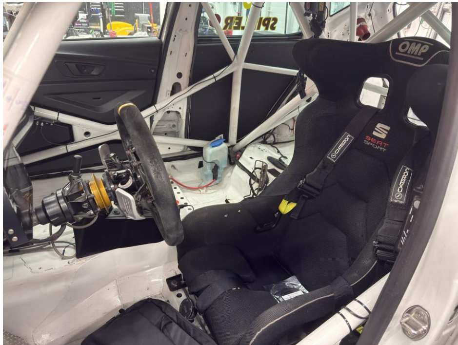
Figure 8 Racing seat, harness and cage members within the modified occupant cell
