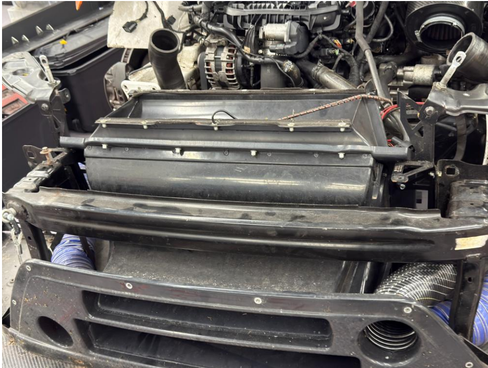
Appendix Figure B1 Front-end support modified to accommodate the race intercooler package
