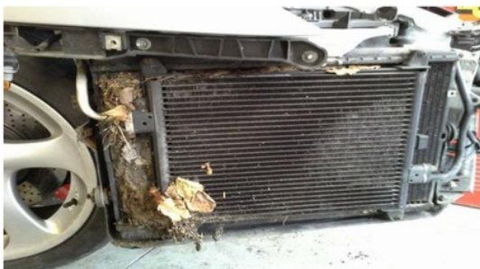
Figure 3 – A design error by Porsche allowing debris to enter through bumper.
