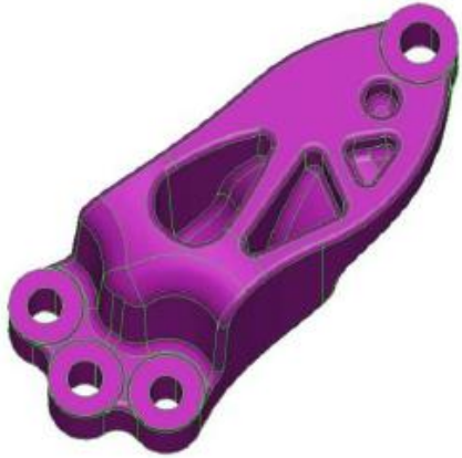
Figure 6. Final optimized CAD manufacture engine mount bracket (Sreedhar & Sasidhar, 2012)
