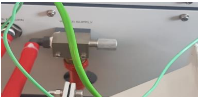
Figure 4 Water Flow Control
