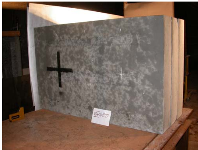
Figure 3. 200 mm thick reinforced concrete wall target
