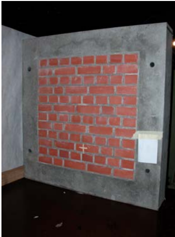
Figure 2. 240 mm thick brick wall target
