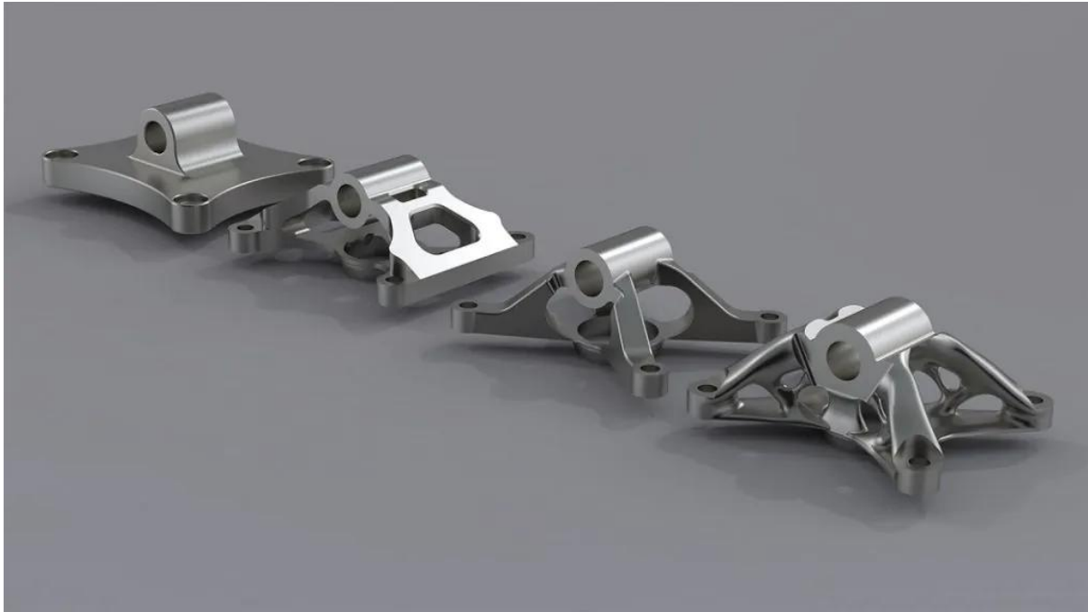
Figure 5 Image showing Generative Design evolution of a component (Source: Sculpteo, n.d: online)
