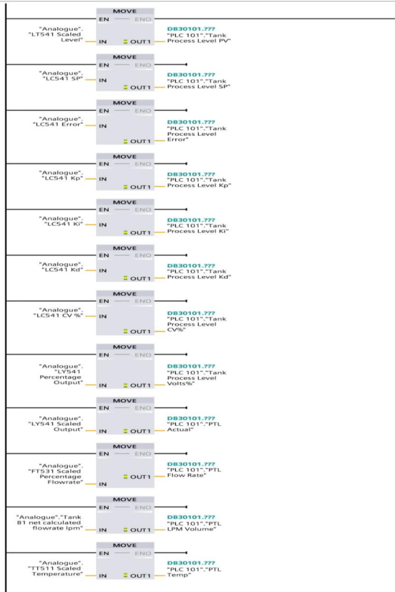
Figure 15;Map Tank level data from PLC 103 to PLC 101. LC541
