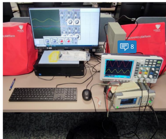
Figure 3 – Virtual and physical signal generator and oscilloscope
