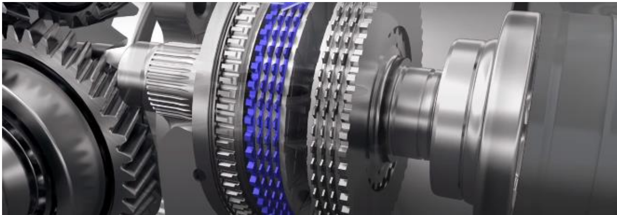
Figure 7-Ferrari FF Clutch pack
