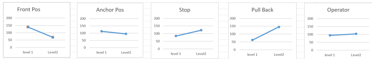
Figure 6: Graphs showing the impact of changing each individual control factor on the distance travelled by the projectile.
