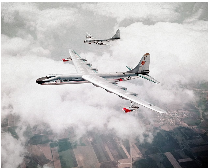
The NB-36H, 1958 — the only US aircraft to ever carry a nuclear reactor. But it only carried the reactor to test the feasibility of the added weight of the reactor and shielding; it didn't power the engines.
