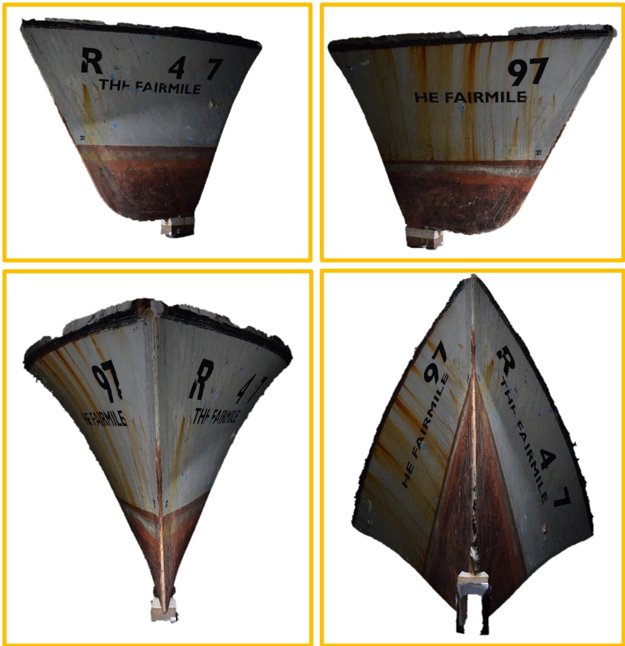
Figure 40: Extracts from photogrammetry model of the bow
