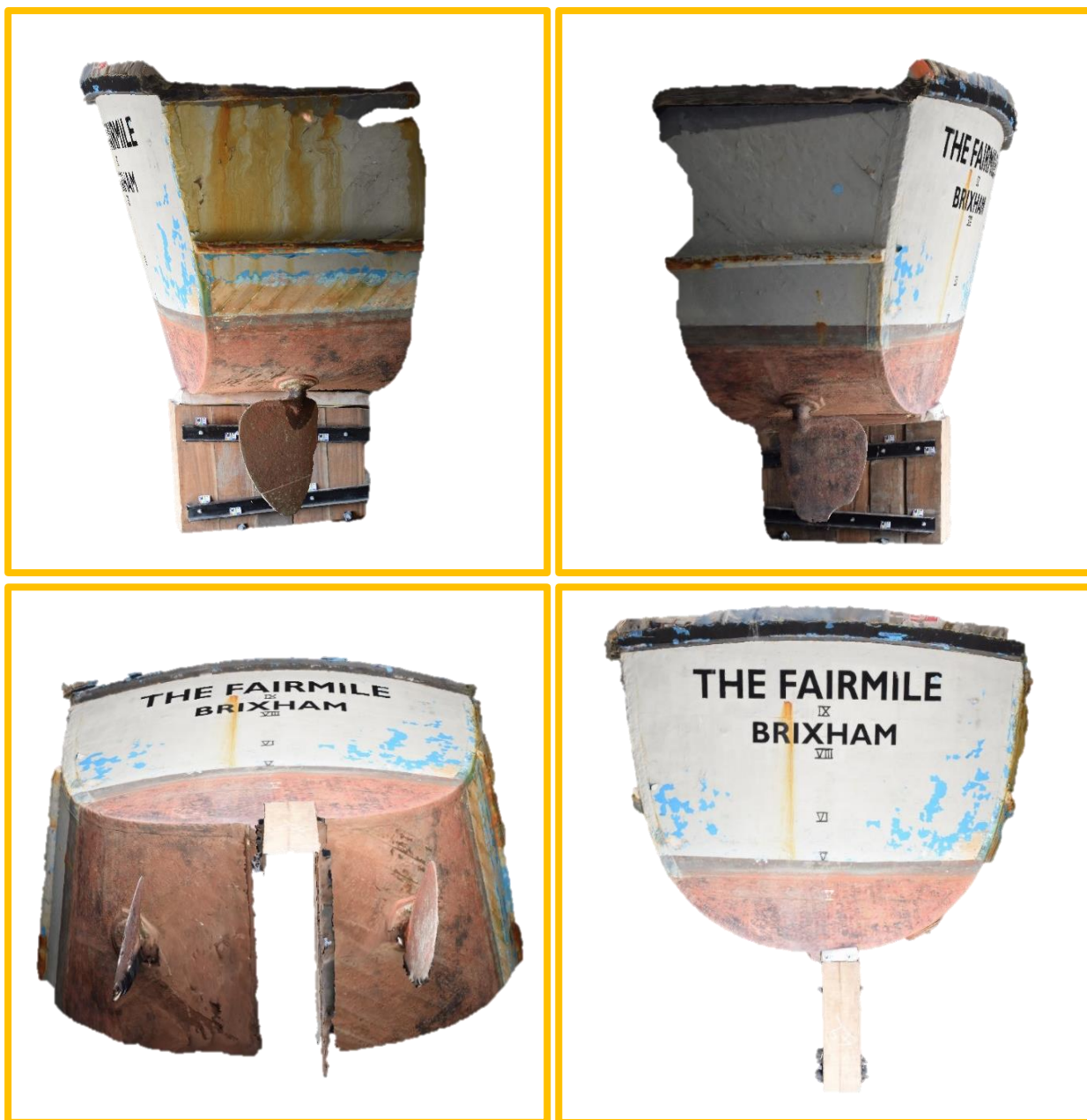
Figure 41: Extracts from photogrammetry model of the stern
