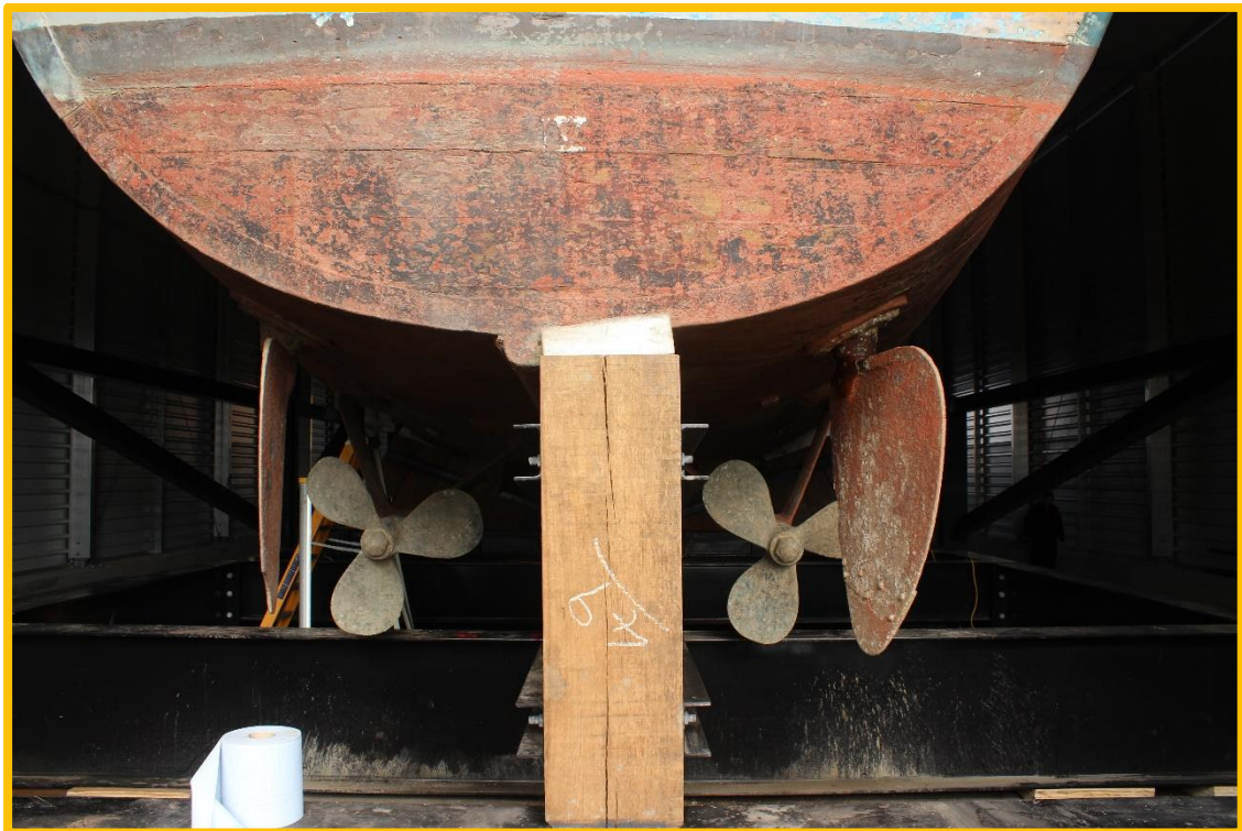
Figure 13: Keel sitting off-centre on the cradle, and cracking in cradle timber
