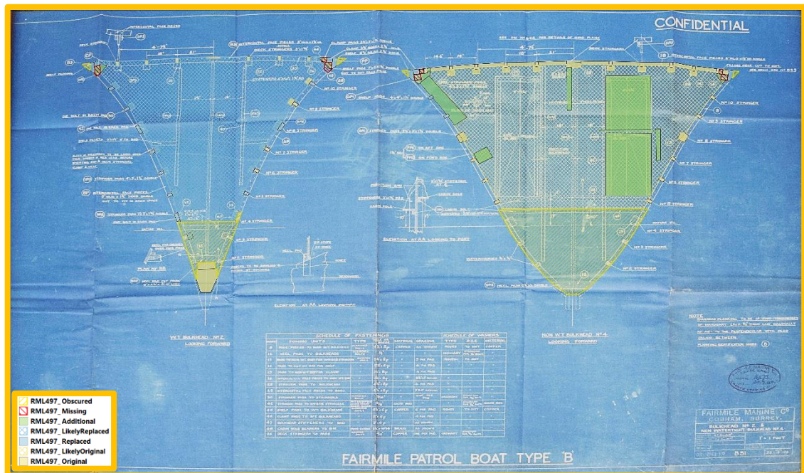
Figure 5: Phasing of bulkheads 2 and 4
