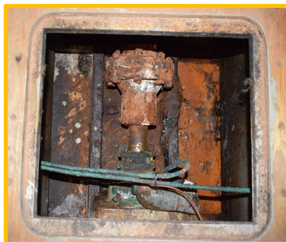
Figure 24: Propeller shafts and greasers below decks in Ward Room
