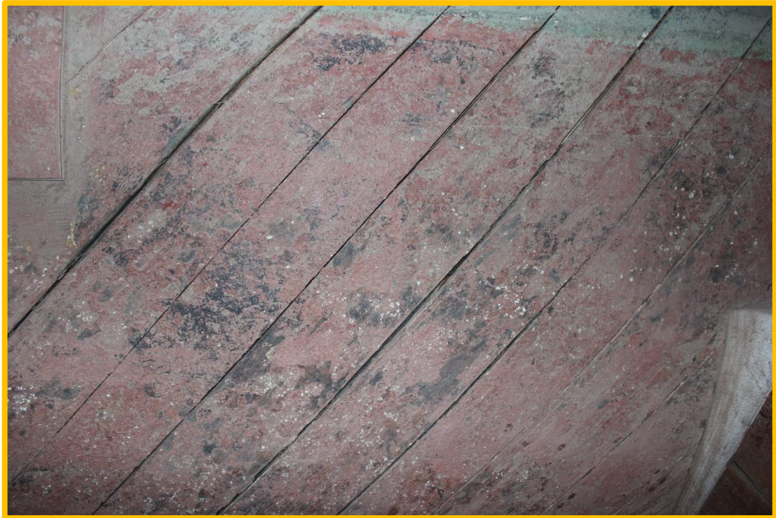
Figure 12: Plank shrinkage on external hull on starboard side close to stern
