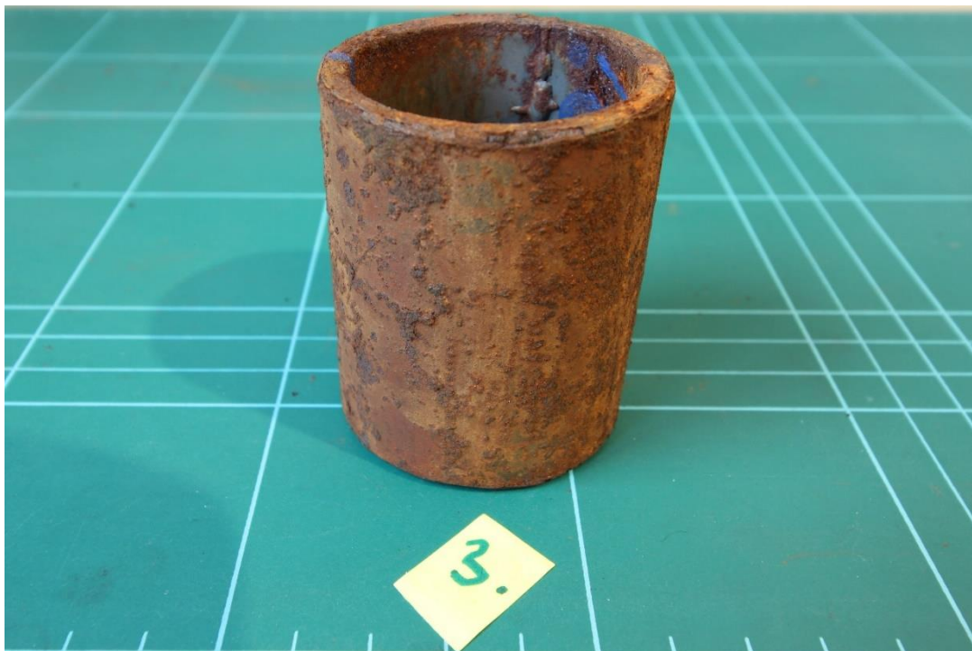
Figure 4.16 Pipe Sample 3 Cyclic – Closed-cell elastomer foam insulation – Coating surface.
