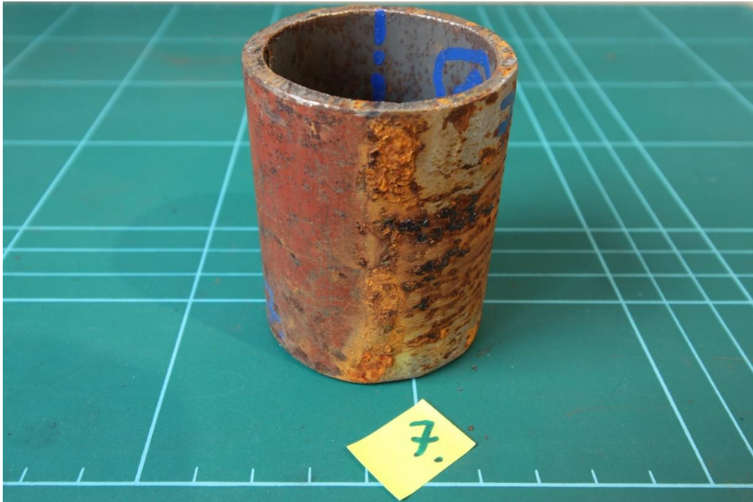
Figure 4.39 Pipe Sample 7 Ambient – Uninsulated - Lower 180°
