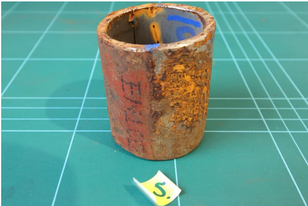
Figure 4.29 Pipe Sample 5 Ambient – Glass wool insulation - Upper 0°
