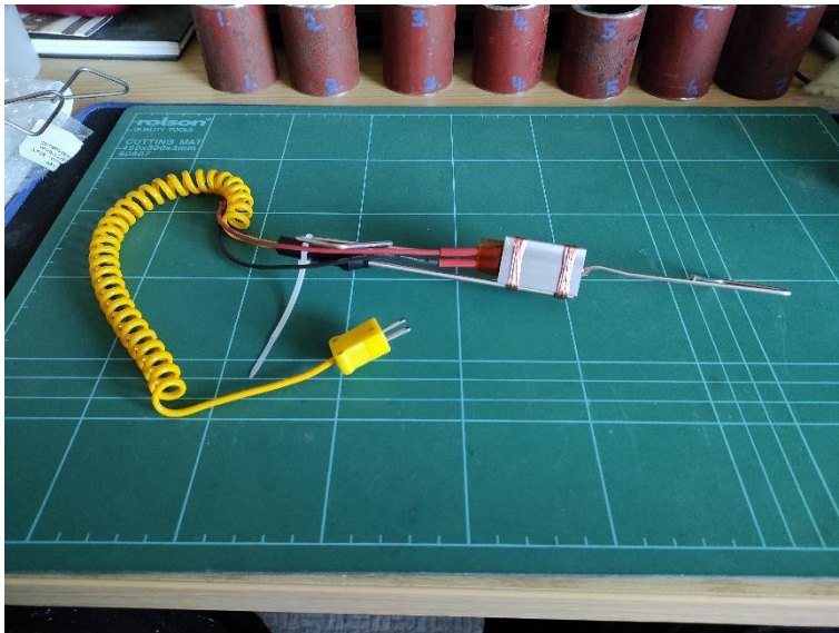
Figure 3.8 PTC element and thermocouple assembly
