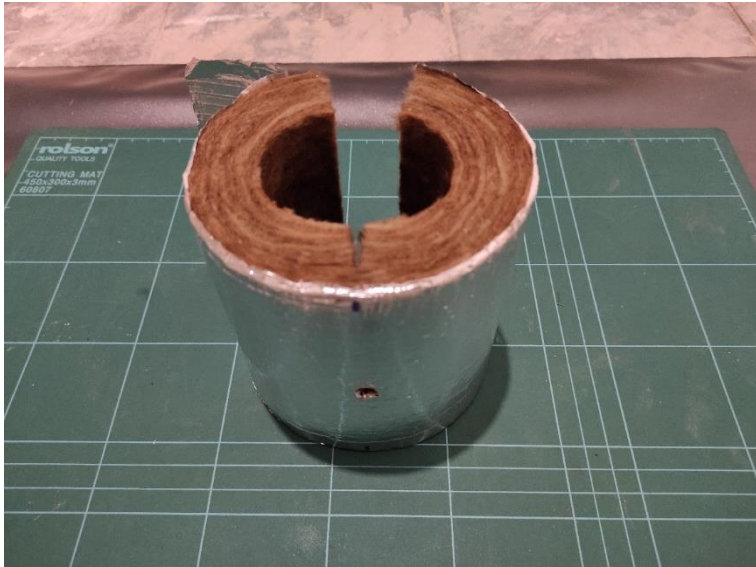
Figure 3.2 Insulation sample preparation, rock mineral fibre shown.
