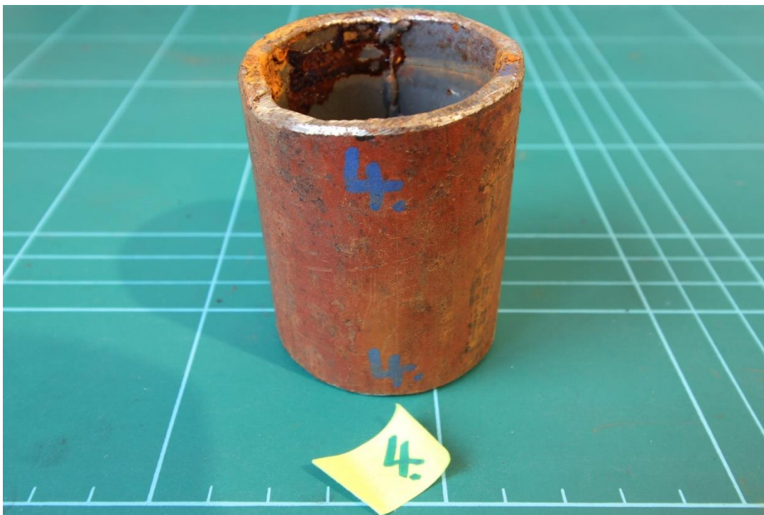
Figure 4.22 Pipe Sample 4 Ambient - Rock Mineral Fibre Insulation – Coating surface.
