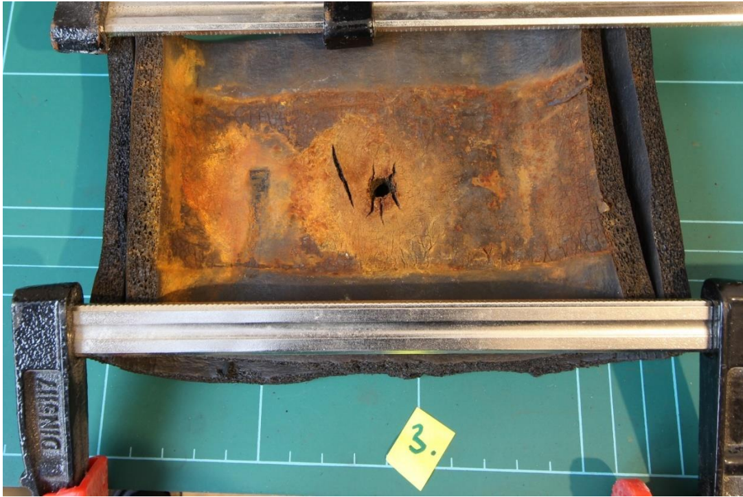
Figure 4.21 Insulation Sample 3 Cyclic – Closed-cell elastomer foam insulation – Inner surface.
