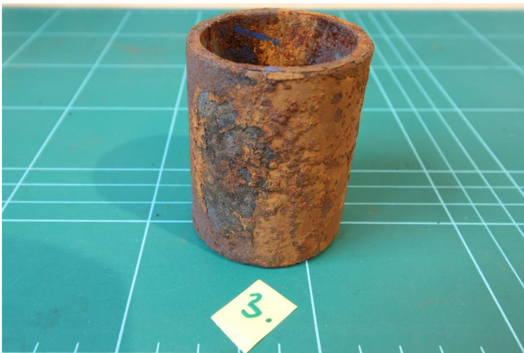
Figure 4.18 Pipe Sample 3 Cyclic – Closed-cell elastomer foam insulation – Upper 0°
