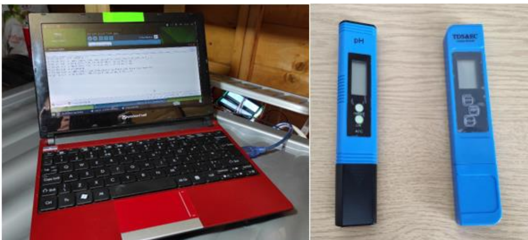
Figure 3.13 Weekly datalogger downloads and water quality measurement instruments
