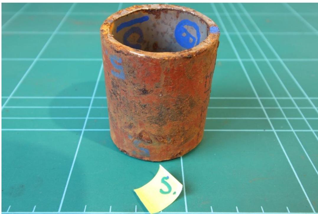
Figure 4.27 Pipe Sample 5 Ambient – Glass wool insulation – Coating surface.
