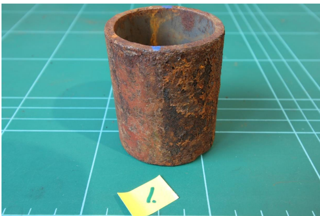
Figure 4.8 Pipe Sample 1 Cyclic – Rock mineral fibre insulation – Upper 0°
