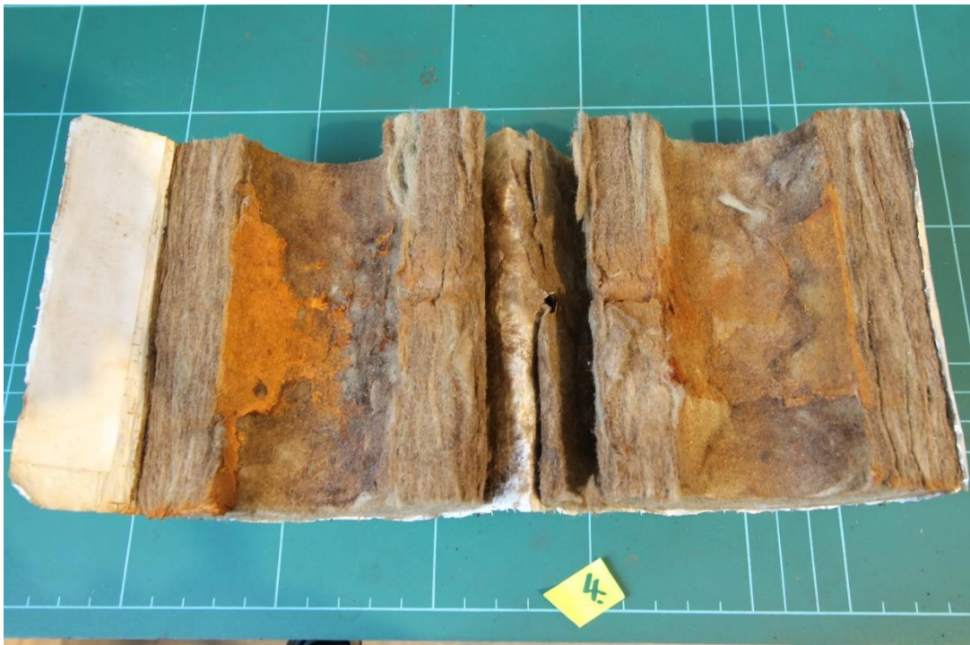
Figure 4.26 Insulation Sample 4 - Rock Mineral Fibre Insulation – Inner surface.
