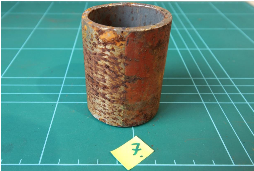
Figure 4.40 Pipe Sample 7 Ambient – Uninsulated - Upper 0°
