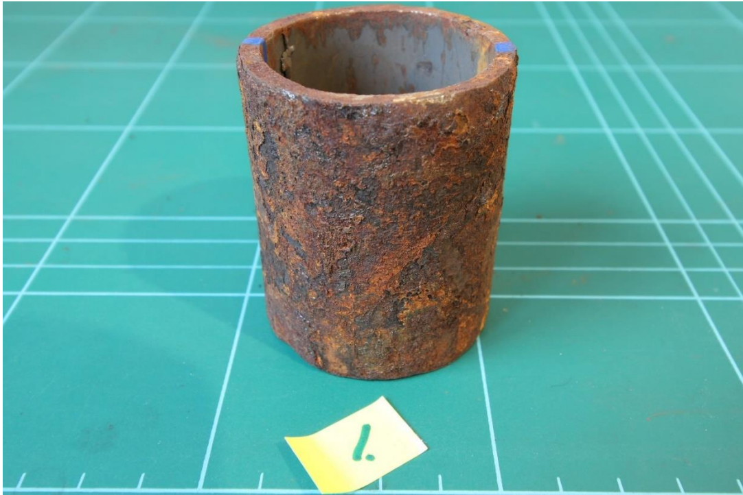
Figure 4.9 Pipe Sample 1 Cyclic - Rock mineral fibre insulation – Preparation surface.
