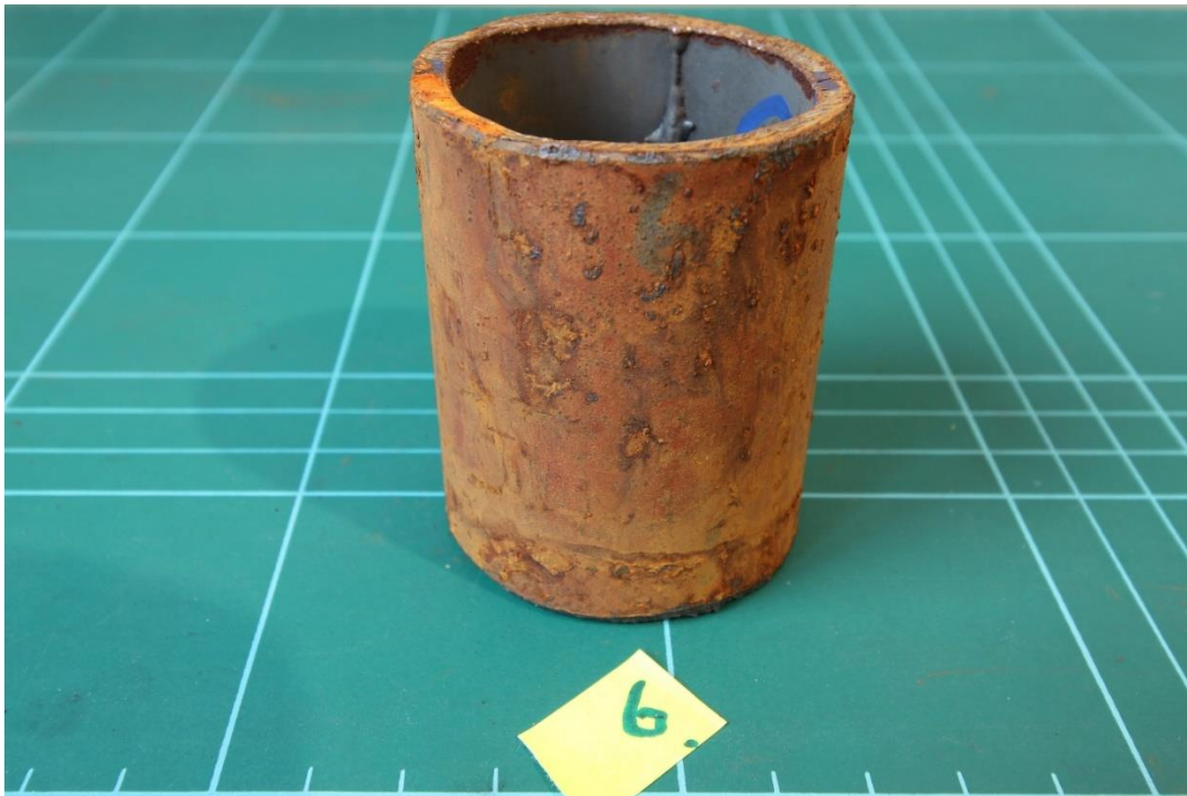
Figure 4.32 Pipe Sample 6 Ambient - Closed-cell elastomer foam insulation – Coating surface.
