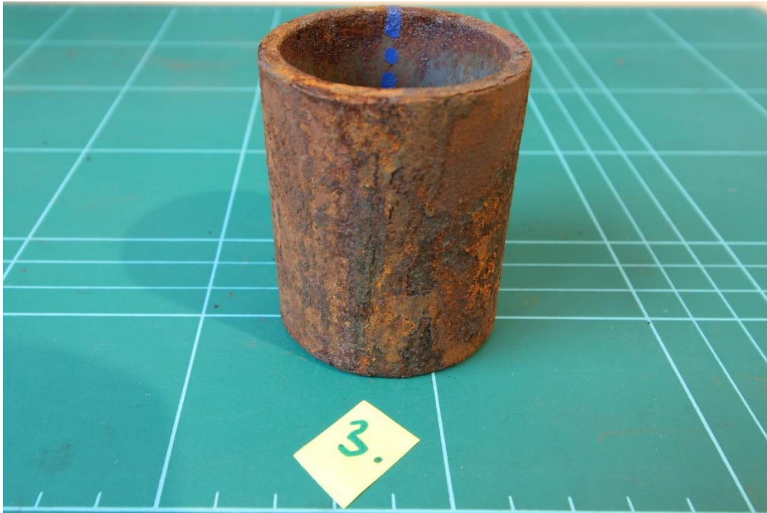
Figure 4.17 Pipe Sample 3 Cyclic – Closed-cell elastomer foam insulation - Lower 180°
