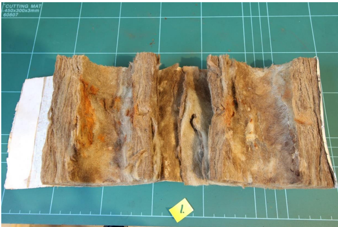
Figure 4.10 Insulation Sample 1 Cyclic - Rock mineral fibre insulation – Inner surface.
