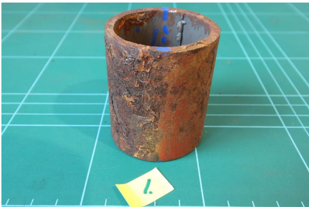
Figure 4.7 Pipe Sample 1 Cyclic – Rock mineral fibre insulation – Lower 180°
