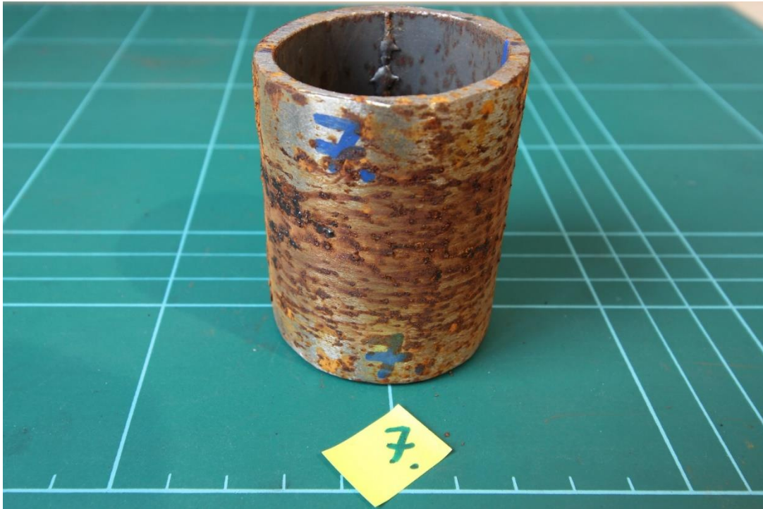
Figure 4.41 Pipe Sample 7 Ambient – Uninsulated – Preparation surface.
