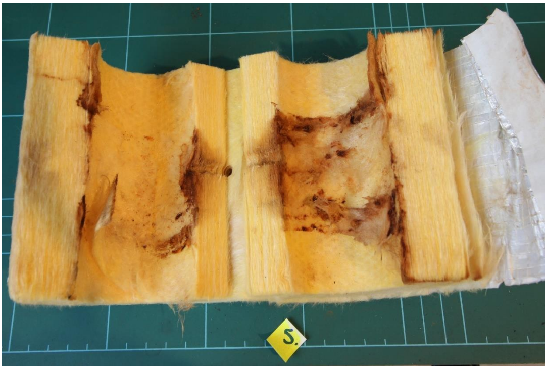
Figure 4.31 Insulation Sample 5 Ambient - Glass wool insulation – Inner surface.
