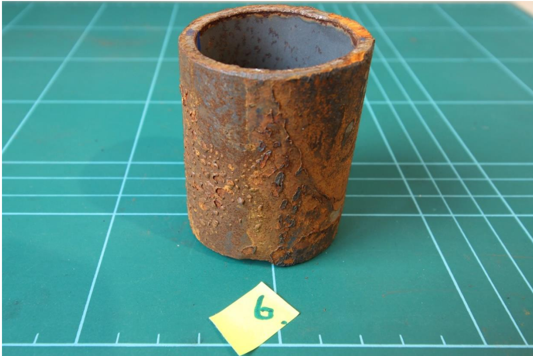
Figure 4.35 Pipe Sample 6 Ambient - Closed-cell elastomer foam insulation – Preparation surface.
