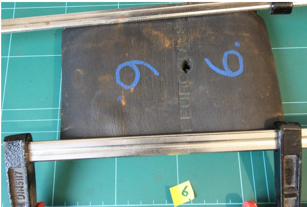
Figure 4.36 Insulation Sample 6 Ambient – Closed-cell elastomer foam insulation – Outer surface.
