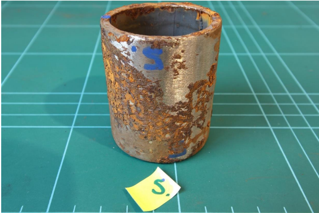
Figure 4.30 Pipe Sample 5 Ambient – Glass wool insulation – Preparation surface.
