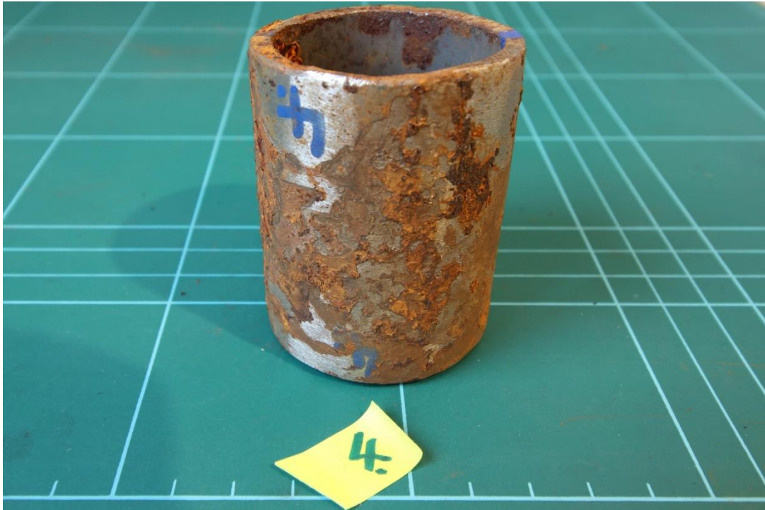
Figure 4.25 Pipe Sample 4 Ambient - Rock Mineral Fibre Insulation – Preparation surface.
