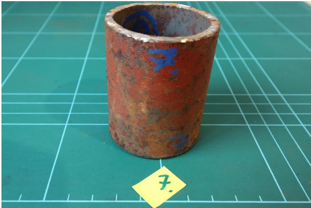
Figure 4.38 Pipe Sample 7 Ambient – Uninsulated – Coating surface.
