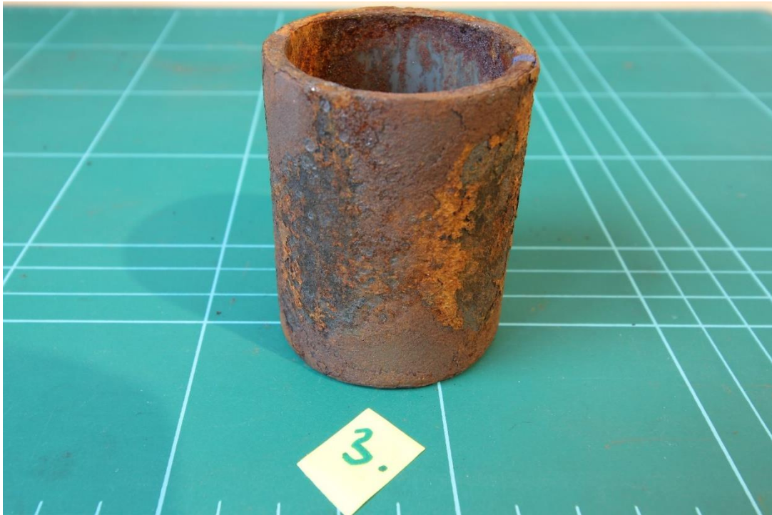
Figure 4.19 Pipe Sample 3 Cyclic – Closed-cell elastomer foam insulation – Preparation surface.
