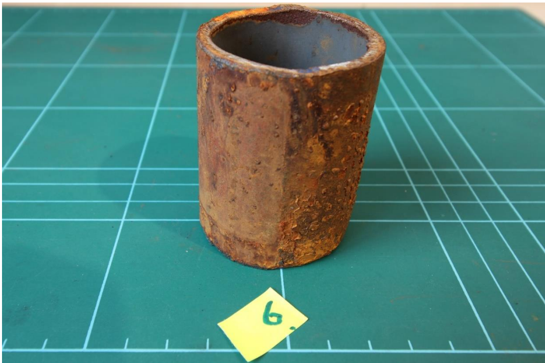
Figure 4.34 Pipe Sample 6 Ambient - Closed-cell elastomer foam insulation - Upper 0°
