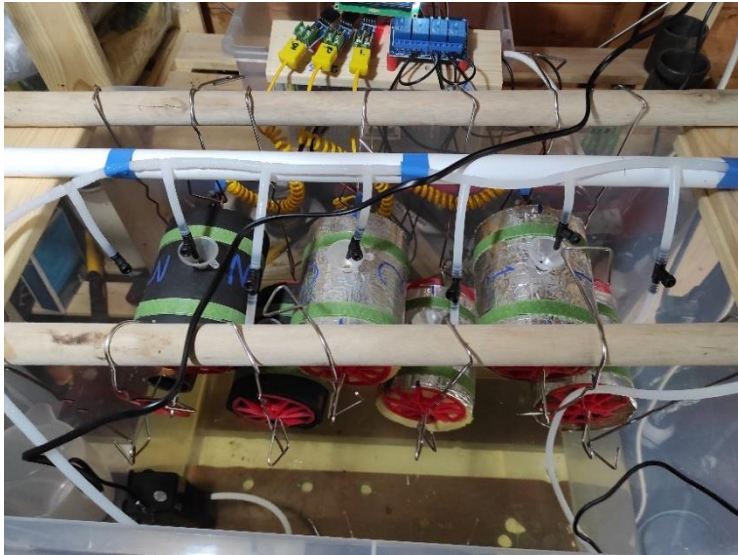
Figure 3.6 Water distribution system in place within environmental tank.
