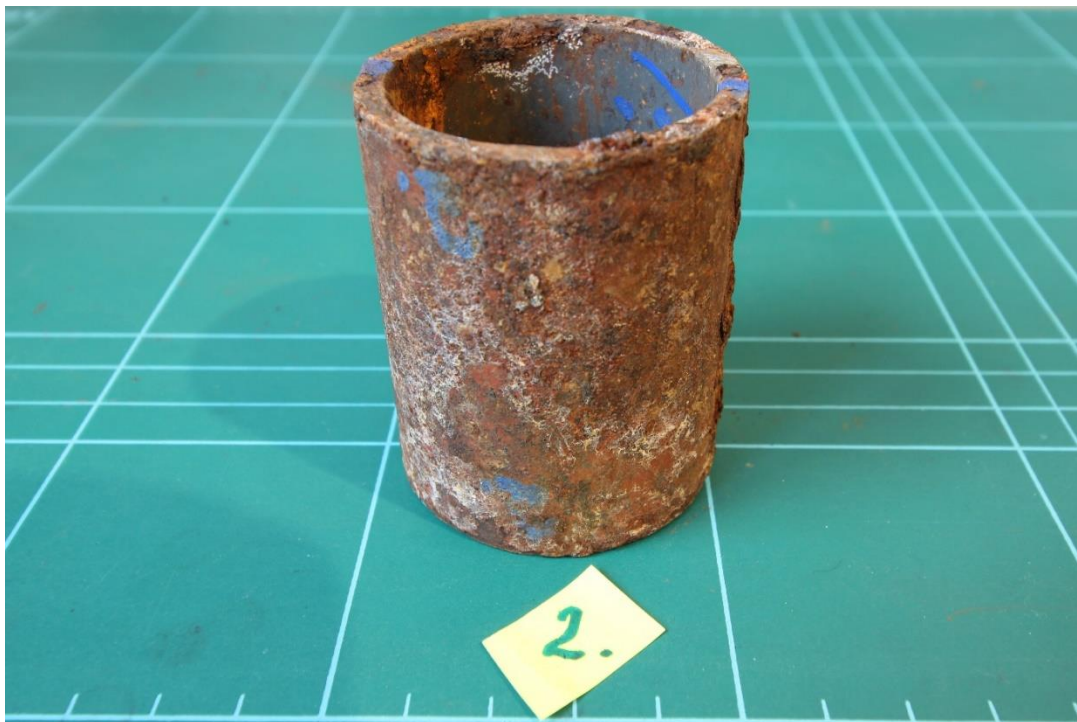
Figure 4.11 Pipe Sample 2 Cyclic – Glass wool insulation – Coating surface.
