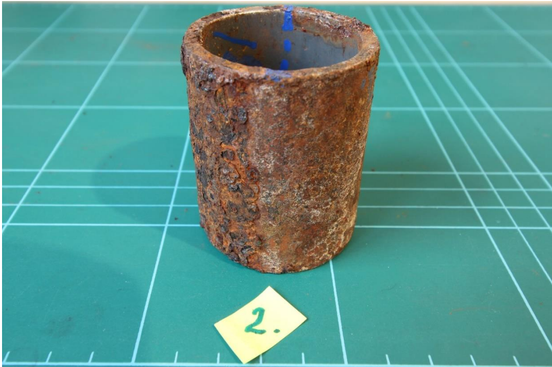
Figure 4.12 Pipe Sample 2 Cyclic – Glass wool insulation - Lower 180°
