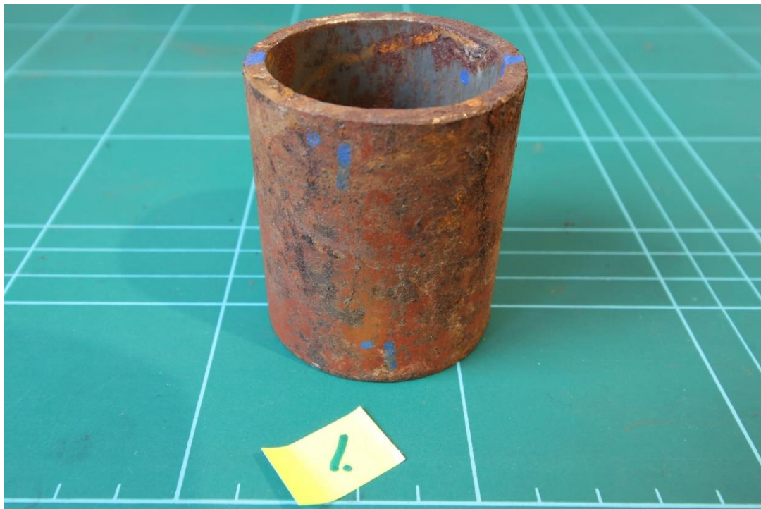
Figure 4.6 Pipe Sample 1 Cyclic – Rock mineral fibre insulation – Coating surface.
