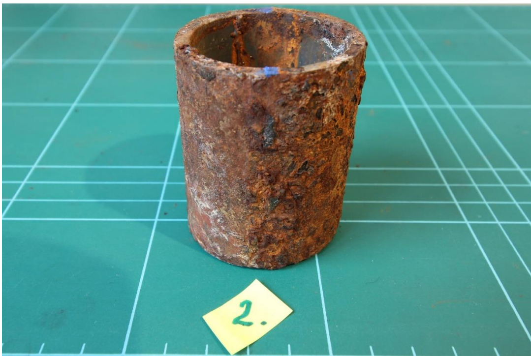
Figure 4.13 Pipe Sample 2 Cyclic – Glass wool insulation - Upper 0°
