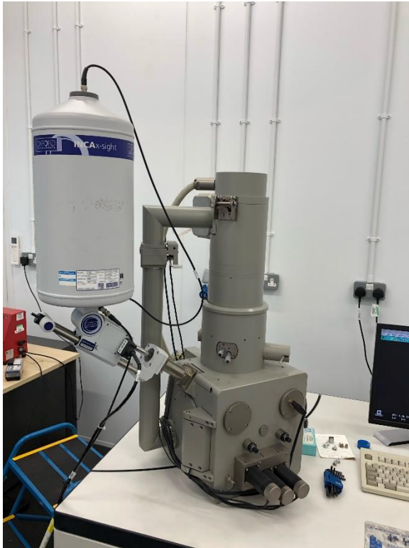
Figure 4.67 SEM and EDX sample chamber
