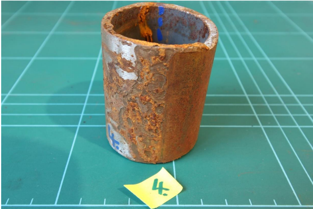
Figure 4.23 Pipe Sample 4 Ambient - Rock Mineral Fibre Insulation - Lower 180°
