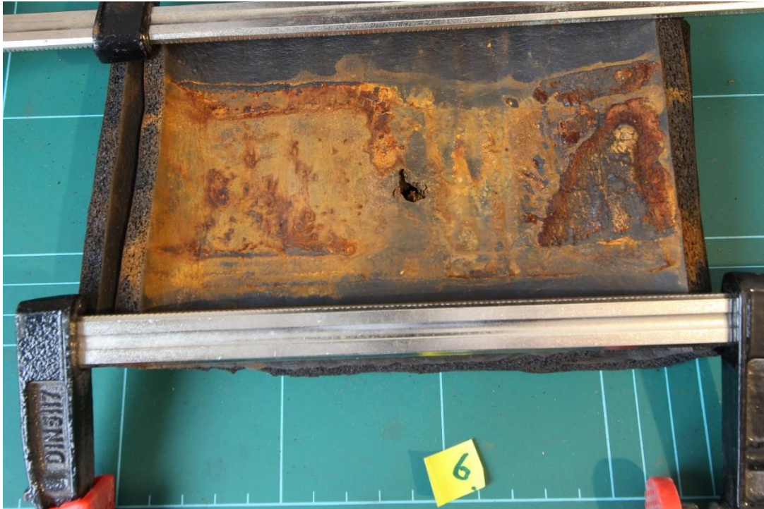
Figure 4.37 Insulation Sample 6 Ambient – Closed-cell elastomer foam insulation – Inner surface.
