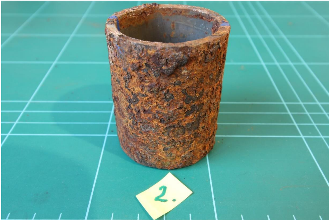
Figure 4.14 Pipe Sample 2 Cyclic – Glass wool insulation - Preparation surface.
