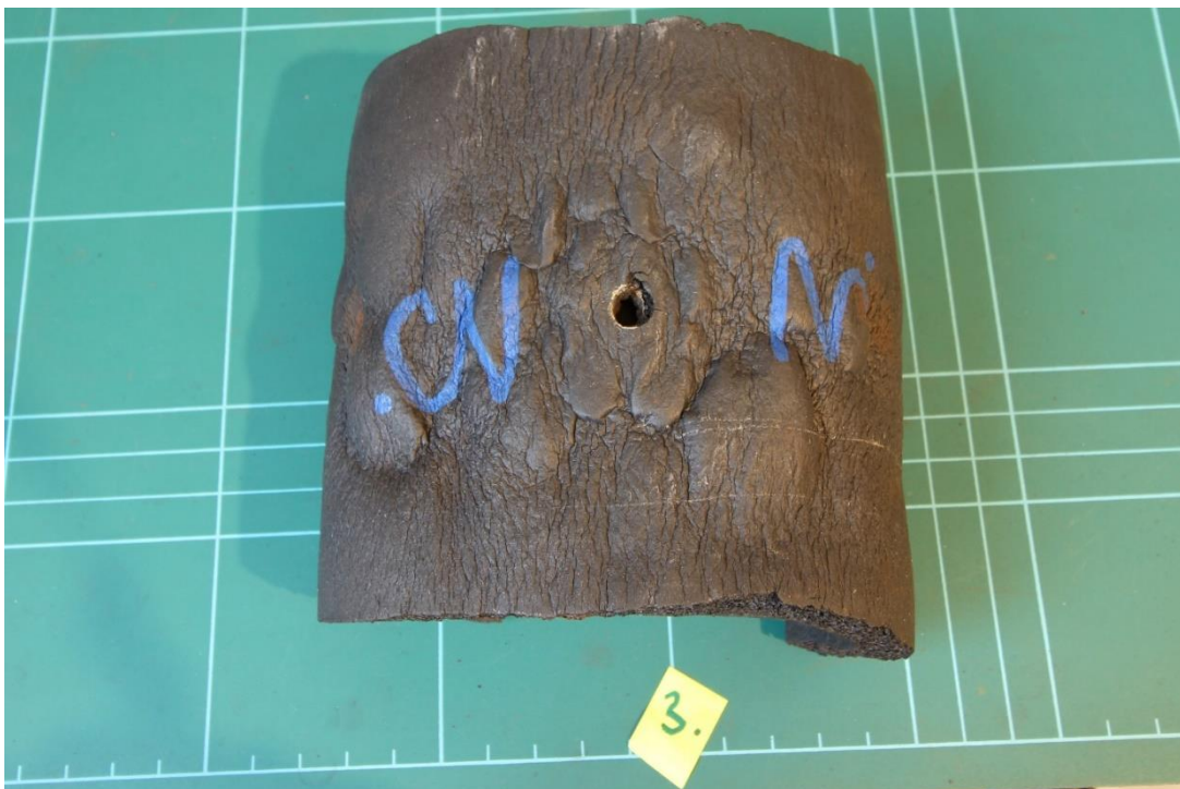
Figure 4.20 Insulation Sample 3 Cyclic – Closed-cell elastomer foam insulation – Outer surface.
