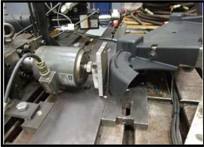
Figure 33 Quasi-static Rear bumper testing
