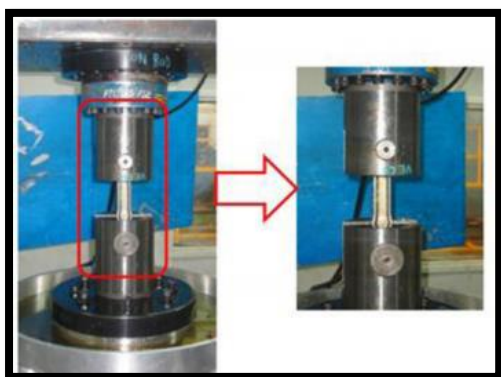
Figure 7 test jig for Fatigue life evaluation
