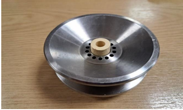
Figure 3:7. Gas Head Insert and Ceramic Molten Metal Guiding Nozzle
