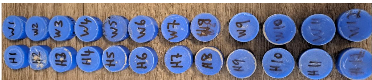
Figure 5:1. Metallography Polished Samples Hybrid & Water Atomized Particles
