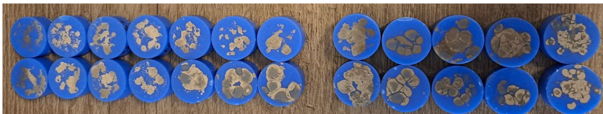
Figure 5:1. Metallography Polished Samples Hybrid & Water Atomized Particles
