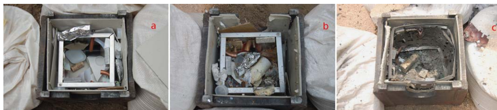
Fig. 2. Container with sample catchers (a) before controlled explosions at AME Pte Ltd. and after (b) low-strength, (c) high-strength explosion with PETN.
