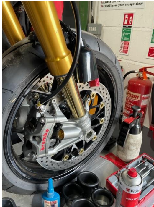
Figure 26 – Front end components installed including Brembo T-Drive discs, braided brake lines, and drilled stainless steel brake calliper mounting bolts.
