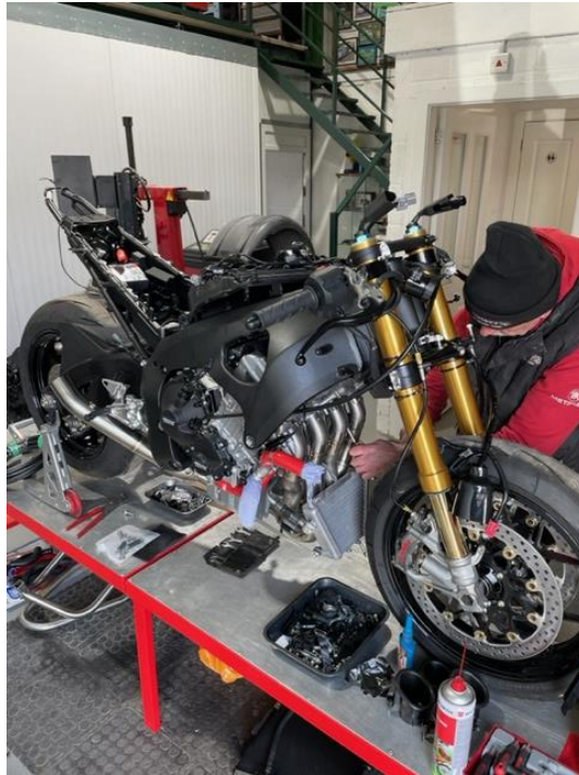
Figure 28 – Exhaust system being installed.
