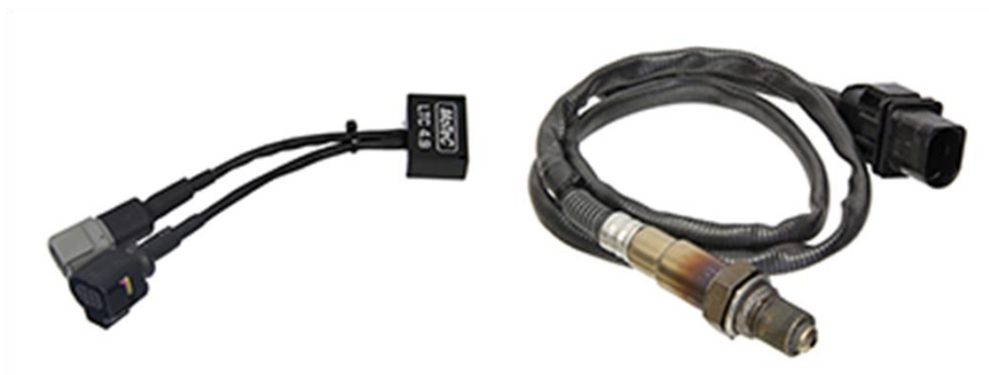
Figure 40 – MoTeC LTC 4.9 lambda measurement unit and lambda sensor used on the project.
