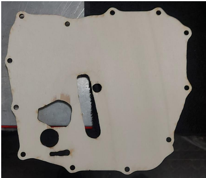
Figure 56 – Prototype baffle plate primarily made for checking hole locations and that there was adequate clearance.
