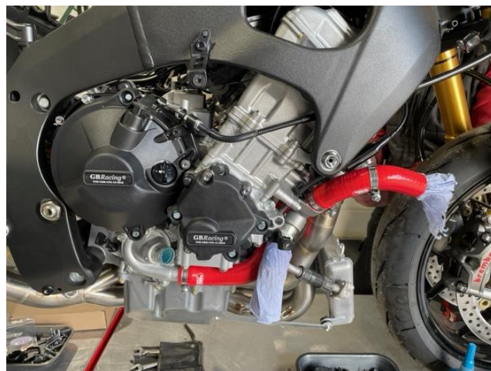
Figure 27 – Engine protection and silicone coolant hoses installed.
