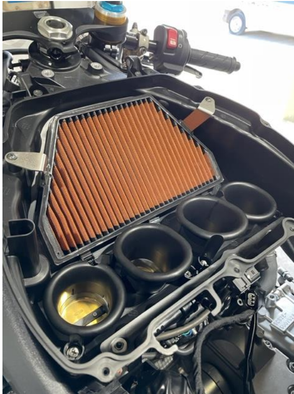
Figure 24 – Sprint aftermarket air filter installed.
