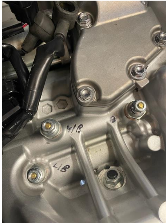
Figure 46 – Three spindle switches located on top of the engine, one for up shift, one for down shift, and one for recognising when the motorcycle is in neutral.
