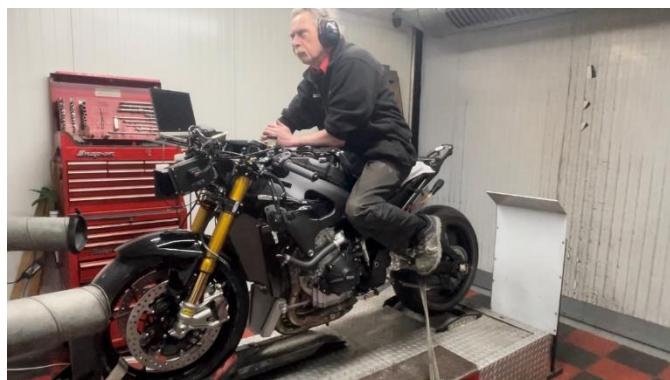
Figure 33 – Running in process on a rolling road dynamometer at Dynobike Performance Tuning in Malton, North Yorkshire.
