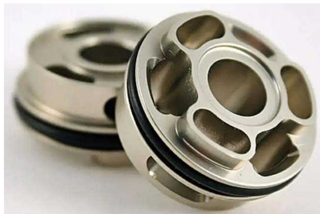
Figure 6 – Piston as found in front and rear suspension units containing orifices that allow oil to pass through them, allowing the suspension to work. [5]
