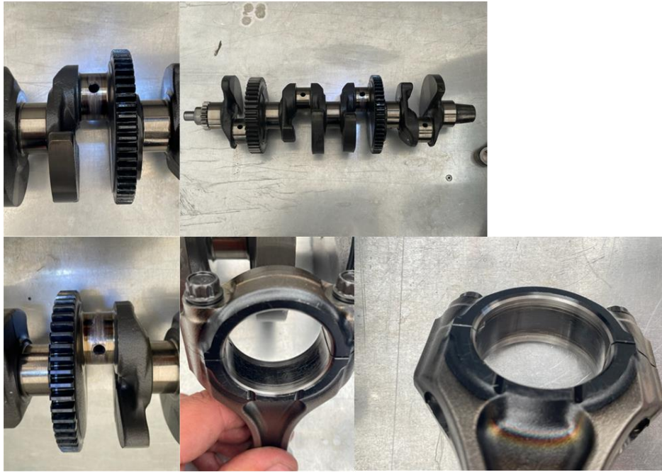
Figure 51 – Broken connecting rod, and crankshaft from the engine failure.
