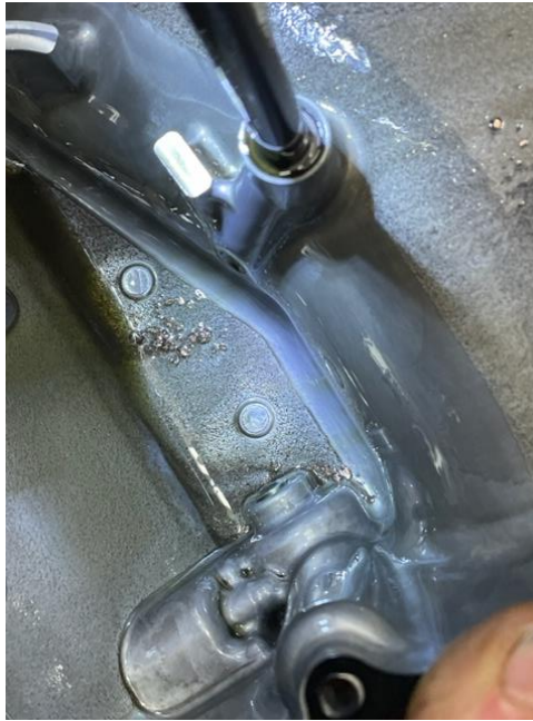
Figure 49 – Small fragments of bronze conrod shell bearing material that was found inside the sump of the engine.
