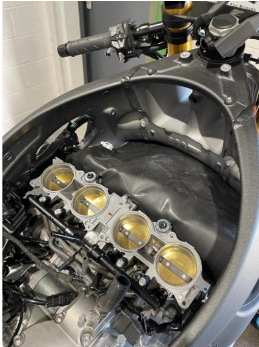
Figure 22 – HRC kit wiring installed and re-installing throttle bodies.
