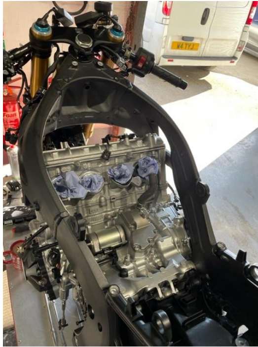
Figure 20 – All wiring and components fully removed and ready to install HRC kit wiring harness.
