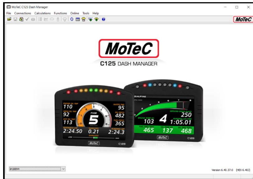
Figure 37 – MoTeC C125 Dash Manager software which was used to control the MoTeC L120 logging system.
